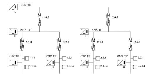
The KNX Coupler has a filter table and thus contributes to reducing the bus load. The filter table (8 kB) supports the extended group address range (main groups 0...31) and is automatically generated by the ETS.
