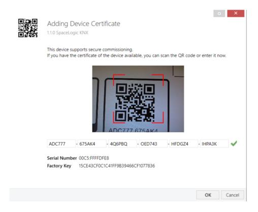
The certificate is printed as text on the device. It can also be conveniently scanned from the printed QR code via a camera connected to the PC that runs the ETS.
