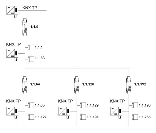
The KNX Coupler can also be used as a repeater. In this case, the individual address has the form x.y.z, where z must not be equal to 0. The filter settings in the parameter dialog of the ETS are ineffective in repeater mode.
