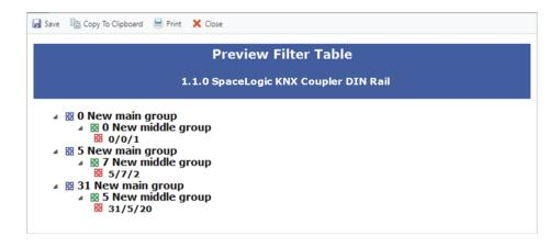
The filter table can be extended by manually adding group addresses. This requires activating "Pass through Line Coupler" in the property window of the corresponding group address.
