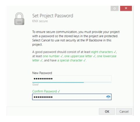
This password protects the ETS project from unauthorized access. This password is not a key that is used for KNX communication. The entry of the password can be bypassed with **Cancel**, but this is not recommended for security reasons.
