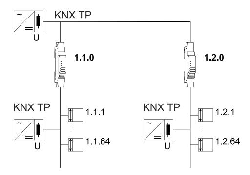
If the individual address is in the form of x.y.0 (x, y: 1...15), the router operates as a line coupler. If it is in the form of x.0.0 (x: 1...15), the coupler acts as a backbone coupler.
