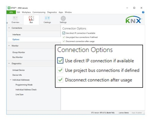
**NOTE:** Due to the significantly shorter transmission times it is recommended to perform downloads via IP.
