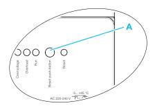
The power supply has a reset button **A**, which, when pressed, shorts the bus line for a defined time or permanently, thus resetting the connected bus devices. It is also possible to acknowledge a fault message via the reset button. Reset the device --> 10
