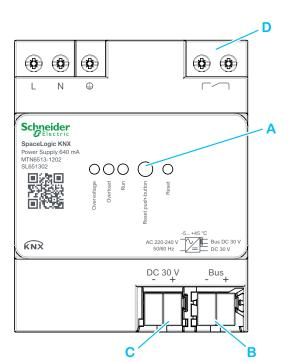
The bus line can be connected to the KNX power supply at connection **B** "Bus". Due to the integrated choke, the use of an external KNX choke is not necessary.
