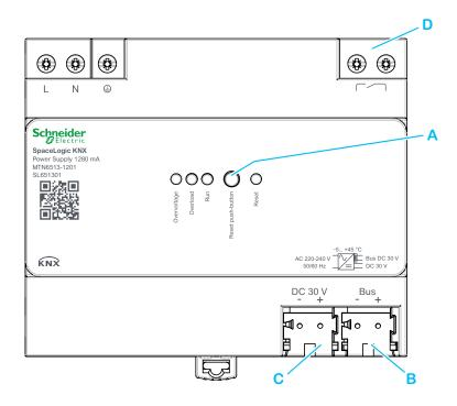
The bus line can be connected to the KNX power supply at connection **B** "Bus". Due to the integrated choke, the use of an external KNX choke is not necessary.
