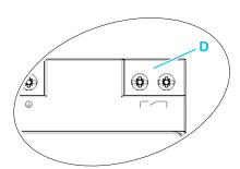
The KNX power supply has a potential-free relay output **D** as a signalling contact for operating or diagnostic messages. This contact is closed in normal operation and open in faulty operation of the devices (overload, overvoltage, KNX voltage failure).Function of the signalling contact --> 12
