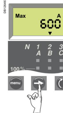
Press the "Arrow" button as many times as required to access the I2 max. screen.
