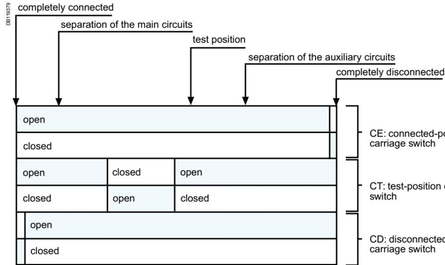
CE: connected-position carriage switch
