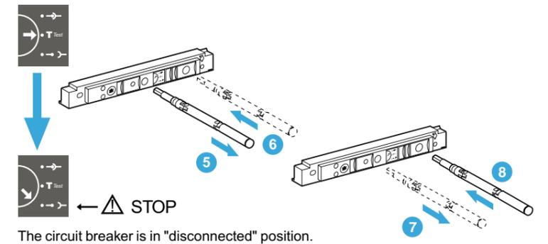
The circuit breaker is in "disconnected" position.
