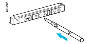
Turn the catch to the right. The circuit breaker can now be locked in all positions.
