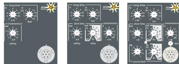
This LED signals that the long-time current setting Ir has been overrun.
