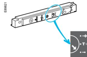
Insert the shackle(max. diameter 5 to 8 mm) of the padlock.
