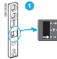
Insert the shackle(max. diameter 5 to 8 mm) of the padlock(s).
