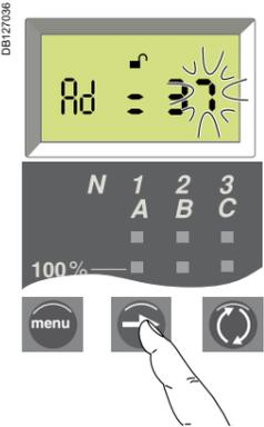
Briefly press the **right arrow** button to display the second digit. The digit will stop flashing and the second digit will start flashing, indicating it is ready to be modified.
