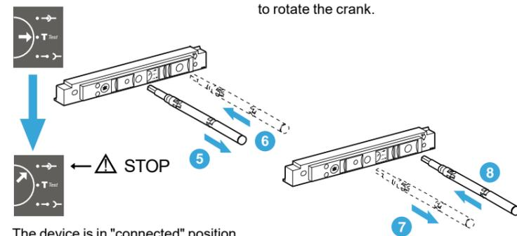
The device is in "connected" position.
