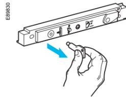
The crank cannot be inserted.
