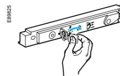
The crank can be inserted.
