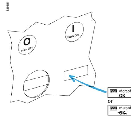
The springs in the circuit breaker operating mechanism must be charged to store the energy required to close the main contacts. The springs may be charged manually using the charging handle or the optional MCH gear motor.
