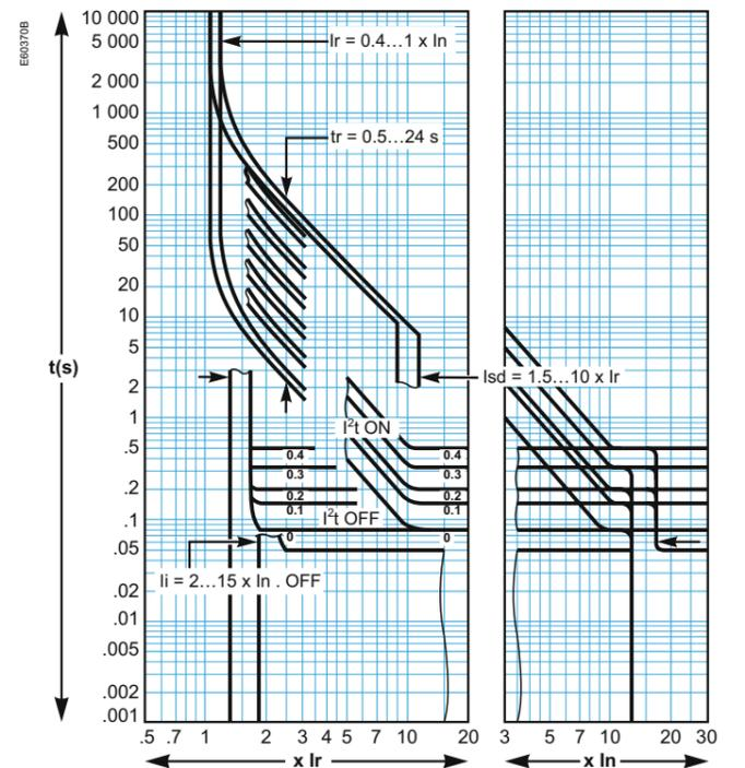
**Long-time, short-time and instantaneous protection (ET/ETA/ETV 6G Trip System)**
