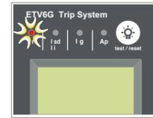
Signals tripping due to an overrun of the short-time pick-up  $I_{sd}$  or the instantaneous pick-up  $I_{si}$  /  $I_i$ .
