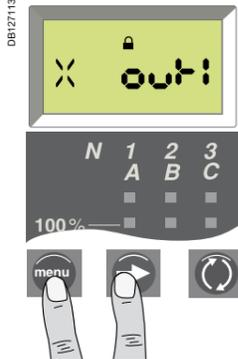
Simultaneously press the **menu** and the **right arrow** buttons for four seconds to access the Modbus address screen. Then press the **menu** button to access the output setting screen. The existing output setting is displayed (default setting is 'X' indicating that no trip event has been assigned to the output). A closed padlock icon indicates that the setting is locked.
