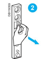
The crank cannot be inserted.
