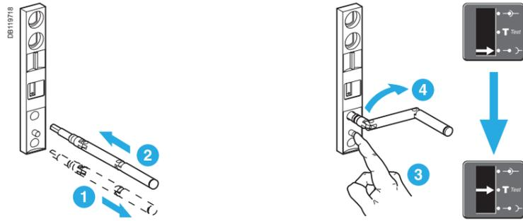
The device is in "test" position.
