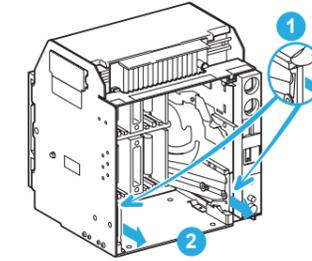
Press the release tabs to push the rails in.
