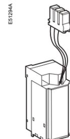
When connected to a remote control panel, the XF closing release (0.85 to 1.1 Un) can be used to close the circuit breaker remotely.
