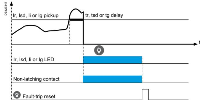
Contact operating diagram for I<sub>r</sub> and I<sub>g</sub> pre-alarms
