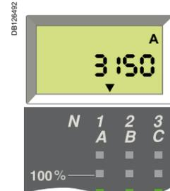
If no particular action is taken, the system displays the instantaneous current of the most heavily loaded phase.
