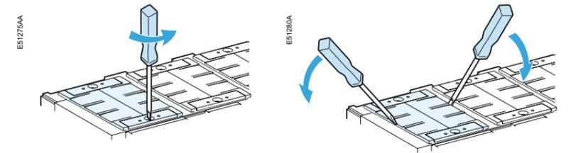
2. check the arc chutes: chamber not cracked separators not corroded.
