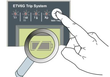
Press the battery-test button (same as the fault-trip reset button) to check the battery status by the luminance of trip indicator light.
