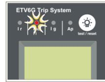
Signals tripping due to an overrun of the ground fault pick-up  $I_g$
