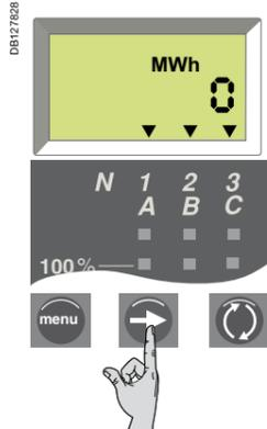
Press and hold the "Arrow" button down for 3 to 4 seconds. The old value changes to the new value (starting at 0) when releasing the button.
