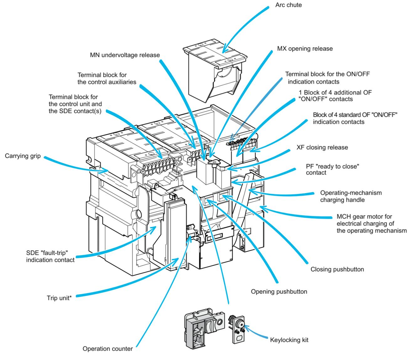
\*Switch-disconnector is supplied without trip unit.
