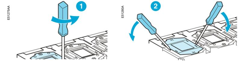
2. check the arc chutes: chamber not cracked separators not corroded.
