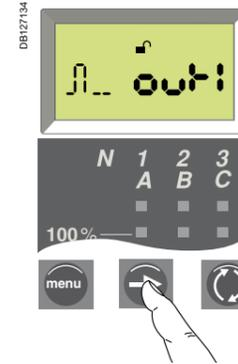
Press on the **right arrow** button to confirm and lock the new setting. The setting stops flashing and a closed padlock is displayed.
