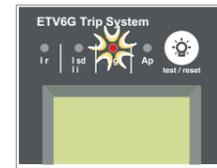
Signals tripping due to the auto-protection, Ap function of the Trip System
