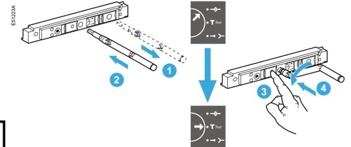
The circuit breaker is in "test" position. Remove the crank or continue to "disconnected" position.
