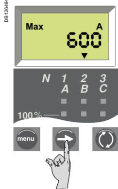
Press and hold the "Arrow" button down for 3 to 4 seconds. The old value changes to the present value (the new maximum).
