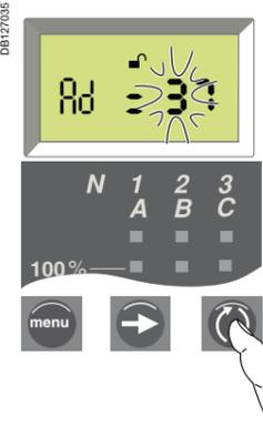
Press the **lock** button repeatedly until the new value for the first digit is displayed. You can scroll through all possible values in a loop<sup>(1)</sup>.
