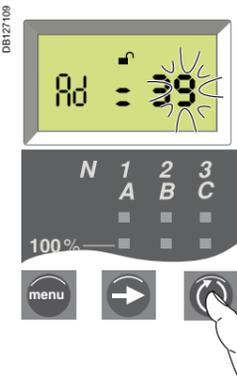
Press on the **lock** button repeatedly until the new value for the second digit is displayed. You can scroll through all possible values in a loop, as for the first digit.
