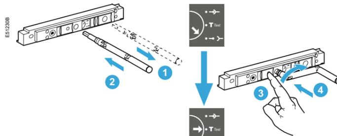
The device is in "test" position. Remove the crank or continue to "connected" position.
