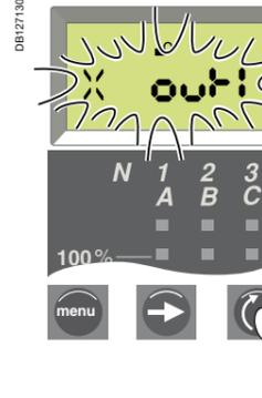
Press the **lock** button to open the padlock. The existing setting will flash, indicating it is ready to be modified.
