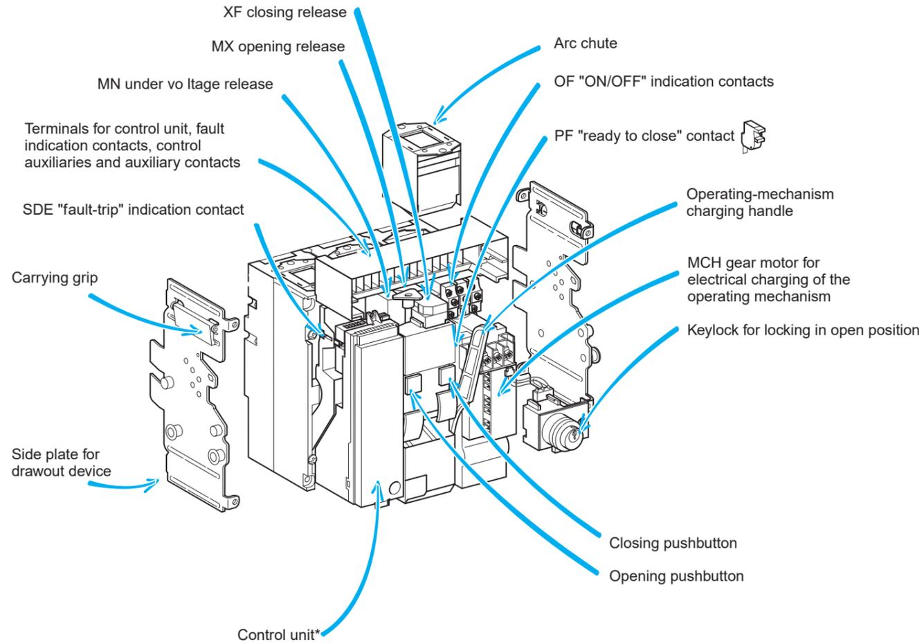
\*Switch-disconnector is supplied without trip unit.
