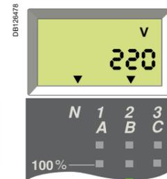
220V phase-to-neutral voltage between phase 2/B and neutral (arrows above N and 2/B).
