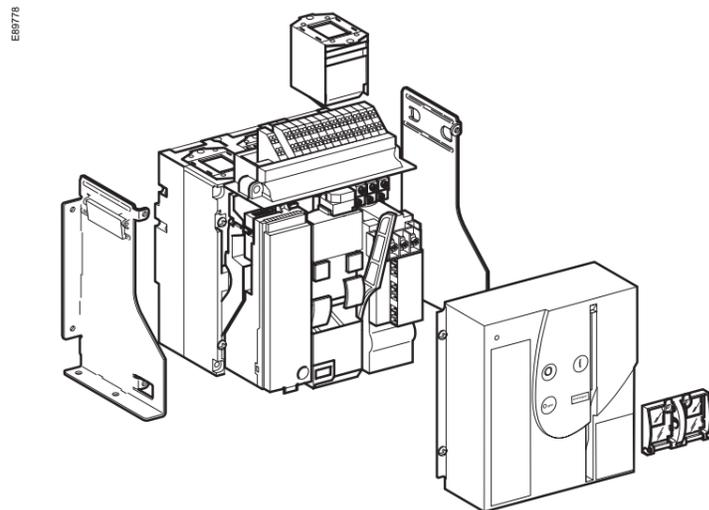
EasyPact MVS circuit breakers are available in drawout and fixed versions. The drawout version is mounted on a chassis and the fixed version is installed using fixing brackets.
