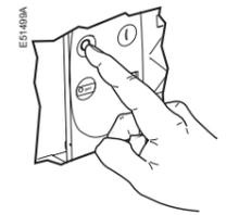
Push the circuit breaker into the chassis, taking care not to push on the control unit.
