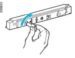
The crank can be inserted.
