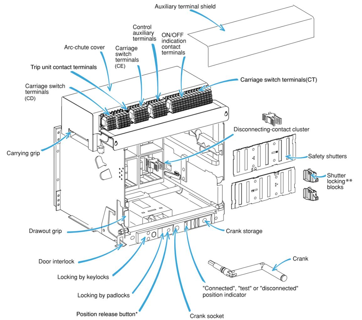
\* During racking-in or racking-out operation of circuit breaker an automatic racking lock button pops out at every distinct position - "Connected", "Test" and "Disconnected". This lock indicates that exact position of the breaker is achieved and blocks operation of the crank. Make sure that the position release button, is pushed-in before rotating the crank.
