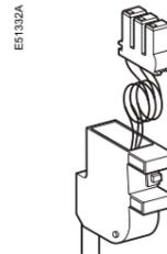
**"Springs charged" limit switch contact (CH)**
