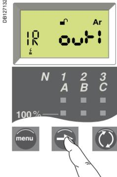
Press the **right arrow** button to confirm and lock the new setting. The setting stops flashing and a closed padlock is displayed.
