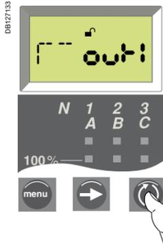
Press the **lock** button repeatedly until the desired output state control mode is displayed (see page 62). In normal mode, the output goes from "0" to "1" (without latching) on occurrence of the assigned event.
