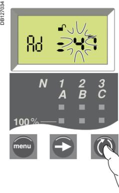
Press the **lock** button to open the padlock and display the first digit (e.g. 4). It will flash, indicating it is ready to be modified.
