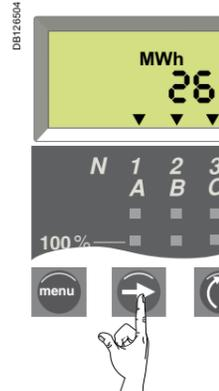
Press the "Arrow" button as many times as required to access the total active energy screen (displaying the whole number part of the total active energy).
