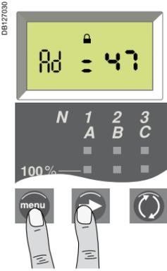
Simultaneously press the **menu** and the **right arrow** buttons for four seconds to access the address setting screen. The existing address is displayed (default address 47 or XX). A closed padlock icon indicates that the value is locked.
