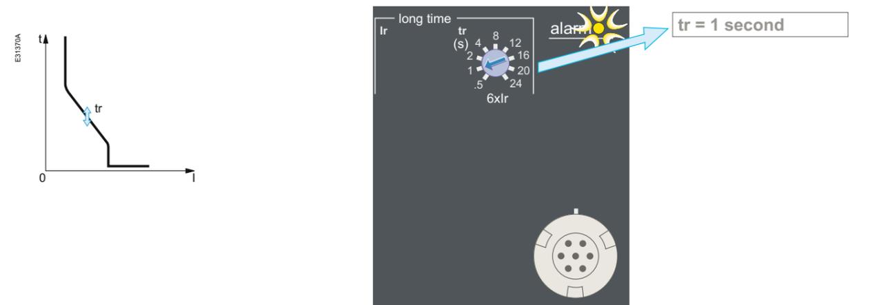
The rating of the circuit breaker in this example is 2000 A.
