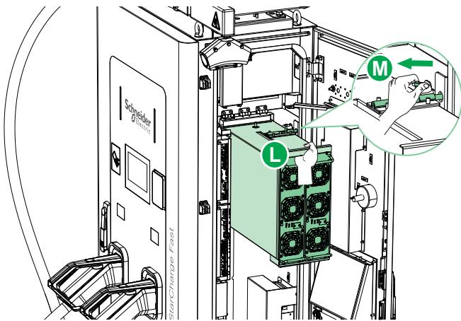
**L, M** • Lift the power module chamber with one hand and unlock the latch with the other hand.
