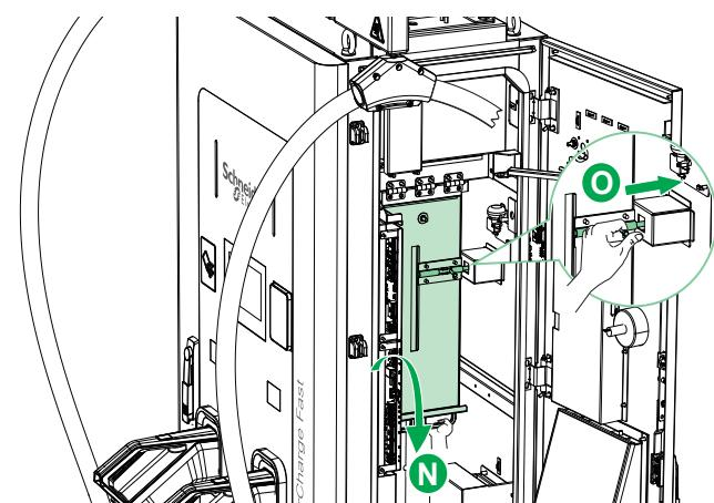
**N, O** • Rotate the power module chamber into place with one hand and lock the latch with the other hand.
