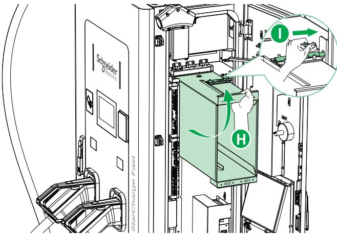
**H, I** • Rotate the chamber and secure the latch.
