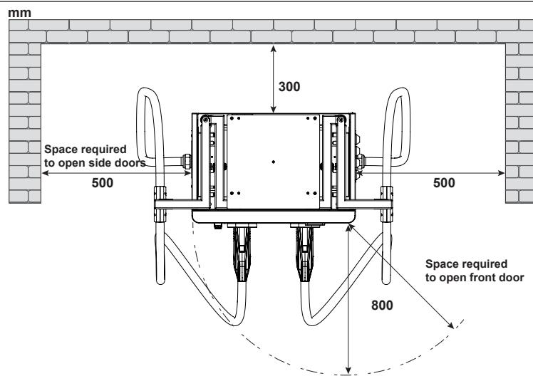
**NOTE:** Ensure that enough space is available around the installation pad to use a forklift and other lifting equipment, unpack crates, remove packing materials, and allow two people to freely move throughout the area.
