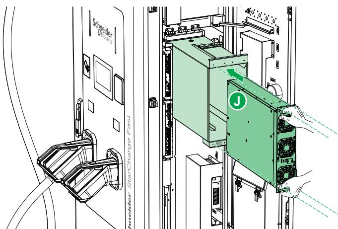
**J** • Carefully with 2 hands hold the power module using both handles and insert in the available slots.
