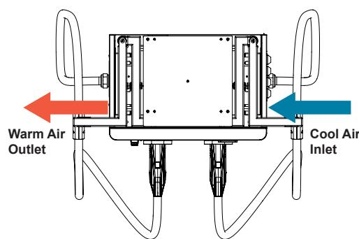
**NOTE:** If necessary, take precautions to prevent snow or objects from blocking the inlets, outlets or the operation of the cable management system.
