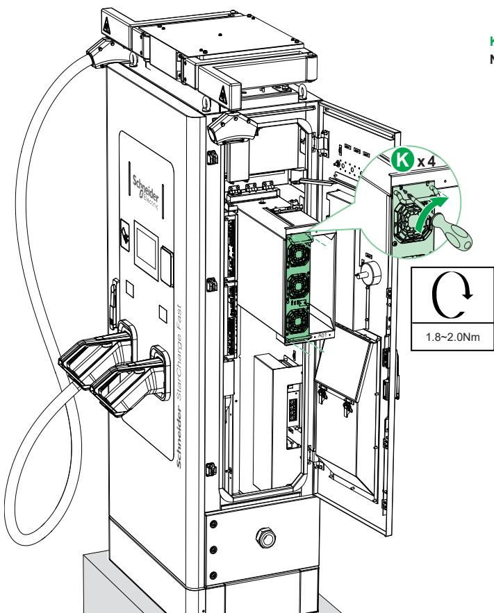
**K** • Use the 4 provided screws to fix the power module in place.
