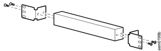
3. Secure the NetBotz 150 to the cabinet, using cage nuts and screws (not provided).
