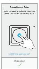
**NOTE:** If the LED is blinking green and red, see the instructions by tapping the link **LED blinking green and red?**.
