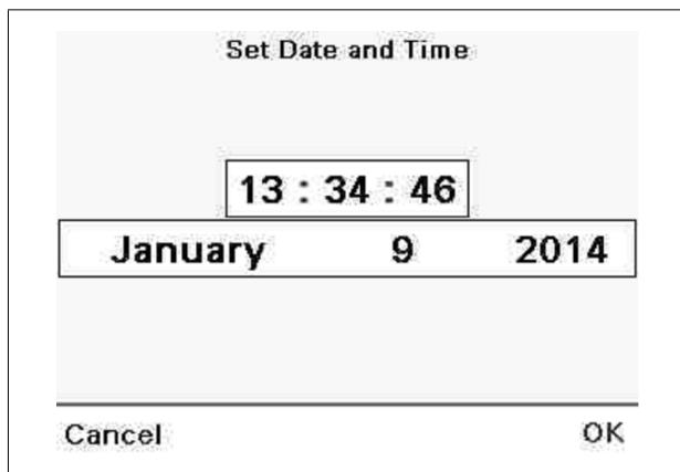
2. Touch the hour, minutes, seconds, date, and year to open a numeric keypad to enter the date and time. Touch the month to display arrows, scroll to the appropriate month and press Enter.
