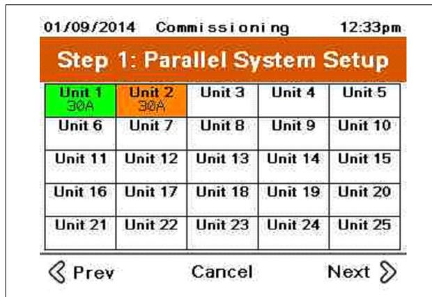
3. By pressing and holding the unit number, a screen will be displayed providing a means to change the unit ID.
