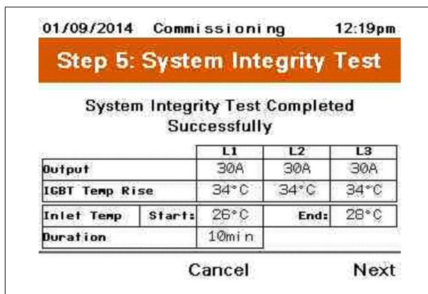
When successfully completed the unit display the output current values per phase, IGBT temperature rise during the test period. The inlet air temperature at the start and end of the test, ant the duration time of the test.
