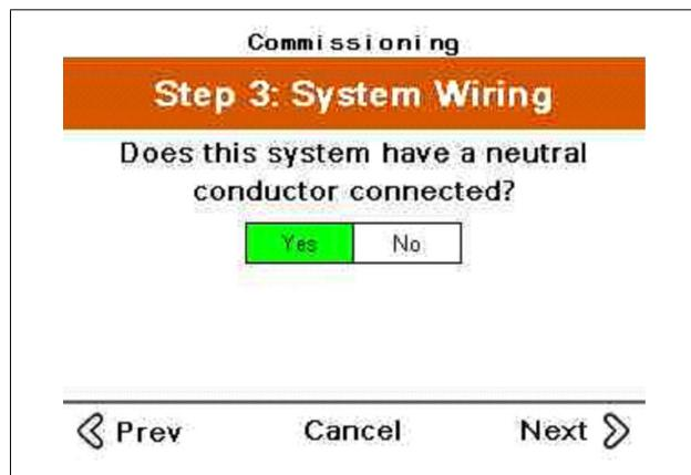
2. Select Yes if a neutral conductor is connected to the system. If a neutral conductor is connected 3 CTs are required to be installed.
