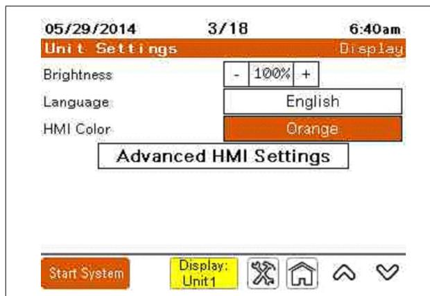
**Brightness:** Press "-" or "+" to adjust the brightness of the HMI display.
