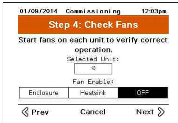
By entering the unit ID number, each fan can be operated for each unit.
