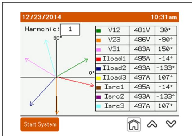
**V12:** Line-to-line voltage of L1 to L2.
