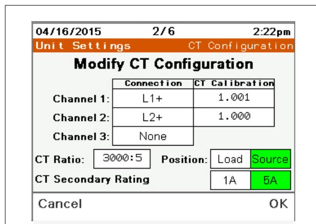
Once the unit is configured for the CTs that are installed, press OK to continue
