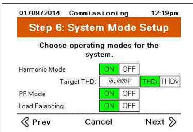
When Harmonic mode is selected, a Target THDi or THDv can be set. Leaving the Target at zero will result in the unit doing the best possible correction.
