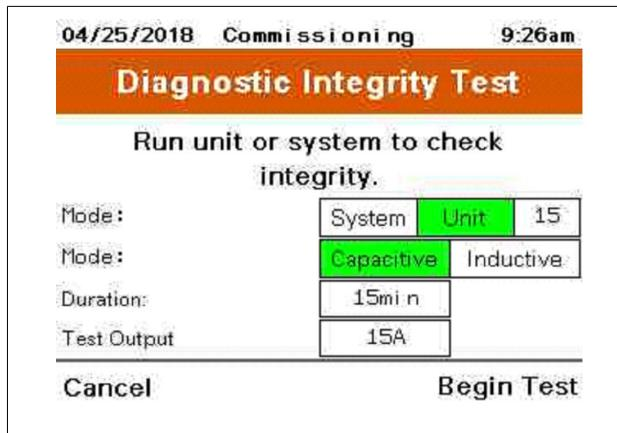
**Mode:** Select system which will cause all units in a system to operate or unit and unit ID to select a specific unit to test.
