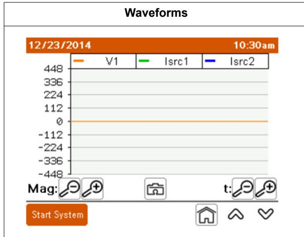
The oscilloscope screen can display up to three different values at the same time. You can touch one of the boxes at the top of the oscilloscope screen to display a table of the 16 different values available.
