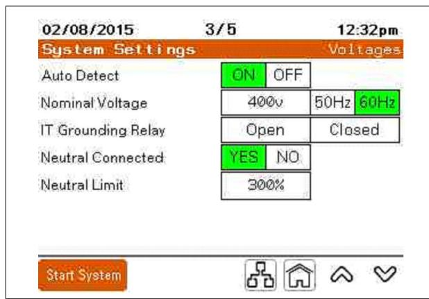
**Auto Detect:** Instructs the controller to determine nominal grid voltage and frequency when power is applied.
