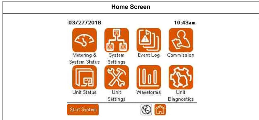
When first energized, the HMI displays the Home screen. To return to the Home screen, press the Home icon at the bottom on any of the screens. To change parameters, you must be logged in as an Admin level user. From the Home screen, you can access the following:
