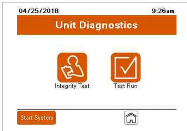
Integrity Test, provides a means to verify the unit or system is operational.
