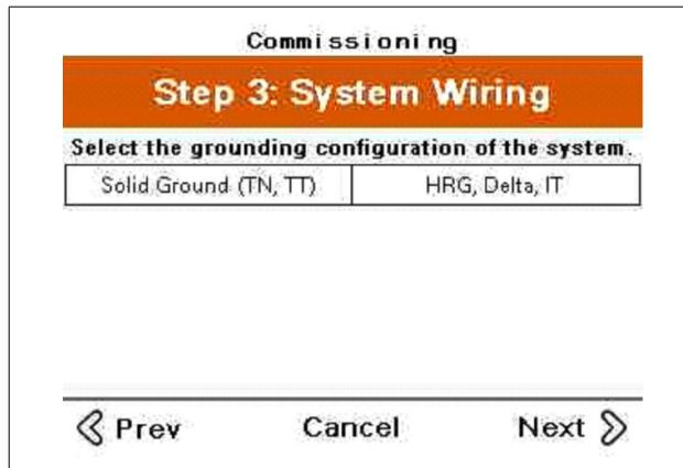
1. Select the grounding configuration of the facility where the system is installed.
