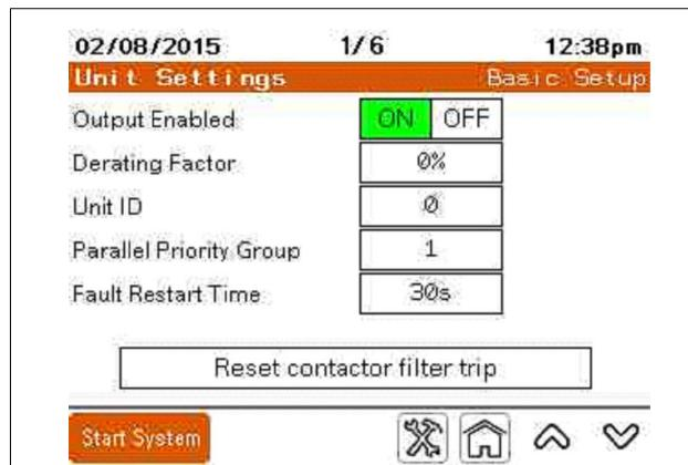
**Output Enabled:** When ON, the unit provides corrective current as necessary. When OFF, the unit does not provide corrective current. Output Enabled must be set to the ON condition after stopping the unit in parallel systems.
