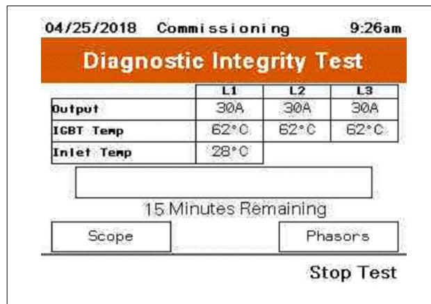
During the test, the HMI will display the output current per phase, IGBT temperature, and unit Inlet temperature during the test. Scope and Phase allows a means to view the oscilloscope or phasor diagram of the unit during operation.
