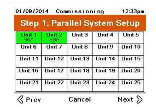
2. For parallel systems, the Parallel System setup screen will be displayed. Pressing the unit ID number will cause the unit number on the screen to cycle in color default is green to orange. The LED on the front of the unit with that ID will also flash.
