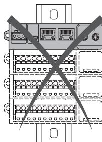
**NOTE:** See the hardware guide for temperature derating when mounting the product other than horizontally.
