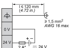
Make the power supply wiring as short as possible.
