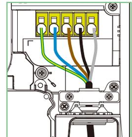
**i** When power supply is single-phase, please follow the wiring method with 1-phase Schneider Charge.
