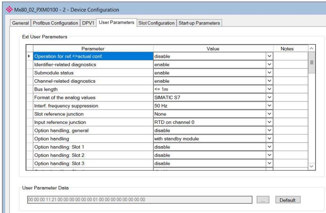
Figure 3.47 – Device User Parameter configuration parameters
