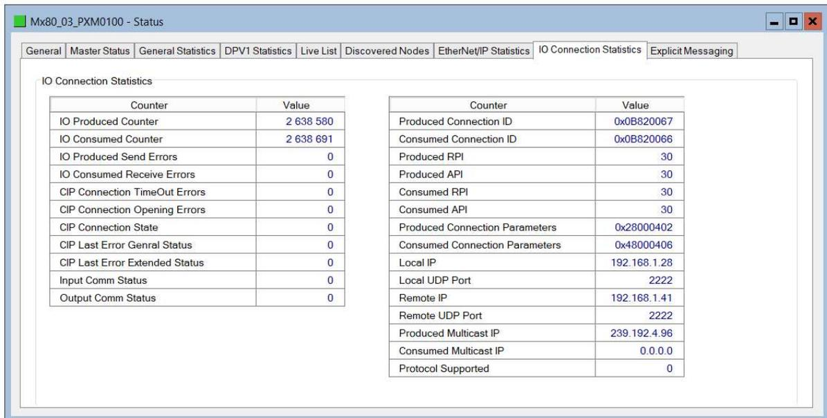
Figure 8.11 – PXM Status monitoring – IO Connection Statistics
