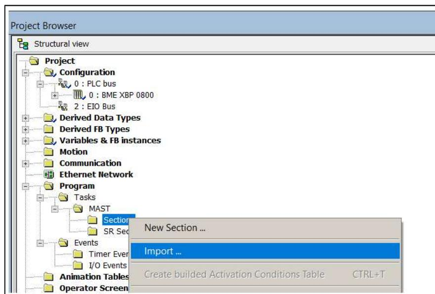
Figure 3.80 – Import Control Expert Mapping from File
