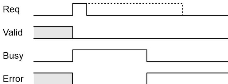
Figure 4.14 – RDRec DFB Timing Diagram - Failure
