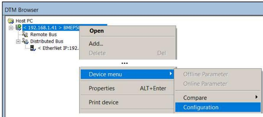
Figure 3.71 – CPU Device Configuration
