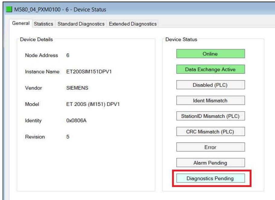
Figure 4.36 – Device Diagnostics Pending in ProSoft Configurator for Modicon
