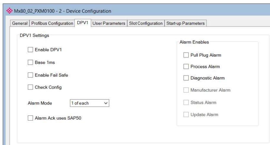
Figure 3.46 – Device DPV1 configuration parameters
