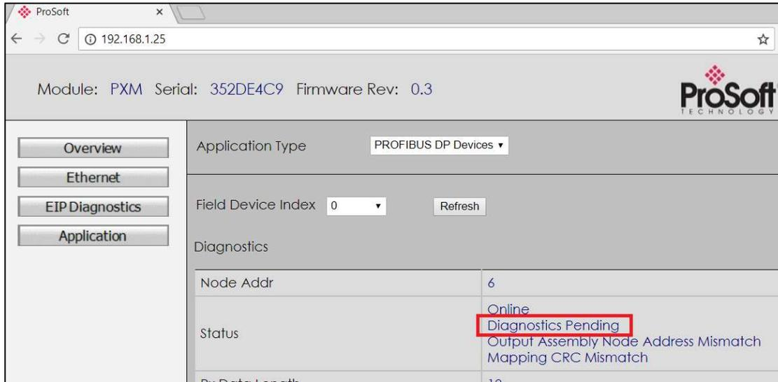
Figure 4.37 – Field device Diagnostics Pending in PXM Webserver
