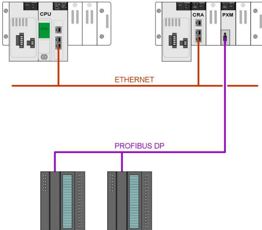
Figure 1.2 - PXM Standalone architecture in a Remote Rack
