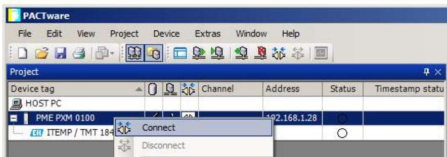
Figure 7.9 – DTM Connect
