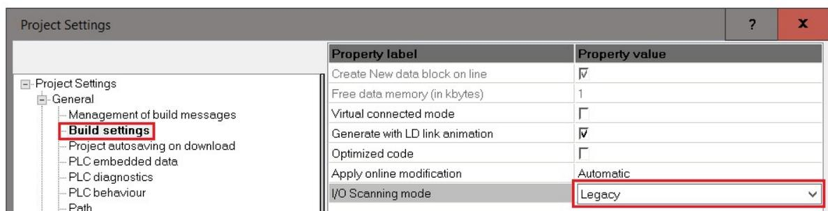
Figure 3.78 – Project Settings – I/O Scanning Mode
