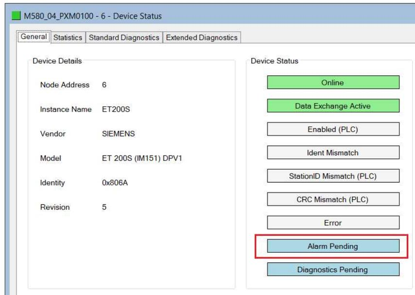
Figure 4.38 – Device Alarm Pending in ProSoft Configurator for Modicon
