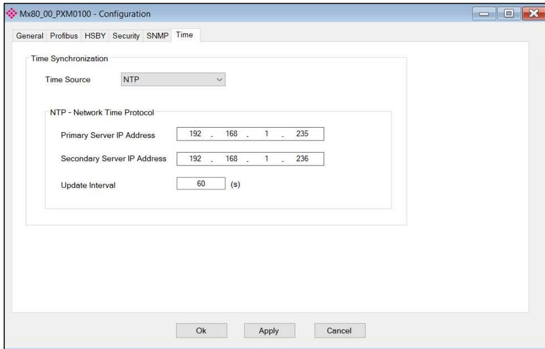
Figure 3.28 – PXM Time configuration
