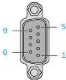
Figure 2.5 - PXM PROFIBUS DP (RS485) DB9 connector
