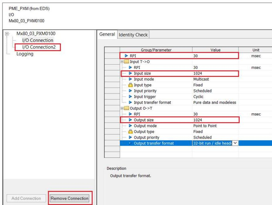
Figure 3.75 – PXM Connection Configuration
