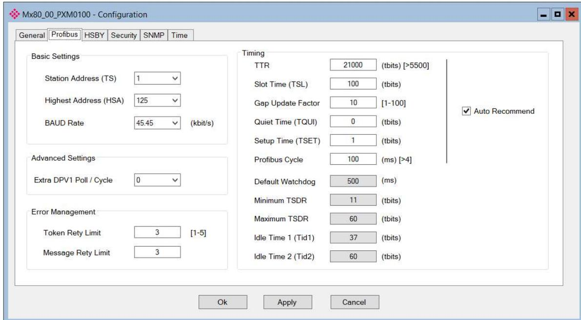
Figure 3.24 – PXM PROFIBUS configuration
