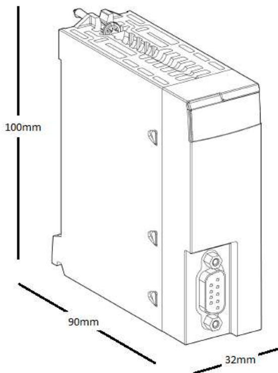
Figure 10.1 - PXM enclosure dimensions
