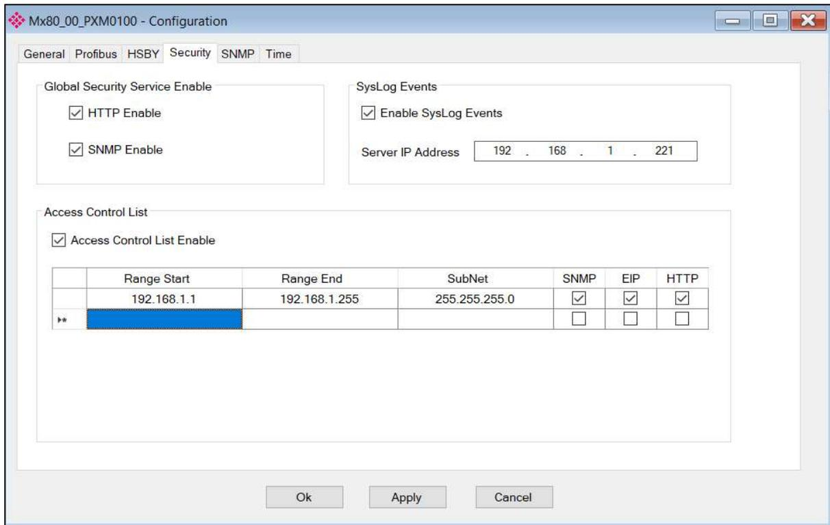
Figure 3.26 – PXM Security configuration
