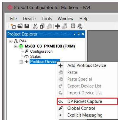
Figure 8.18 - Selecting PROFIBUS Packet Capture
