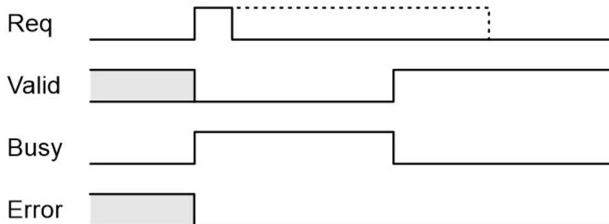
Figure 4.25 – RDAIarm DFB Timing Diagram - Success
