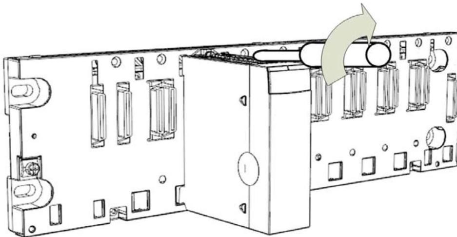
Figure 2.4 – Tightening the PXM to the backplane
