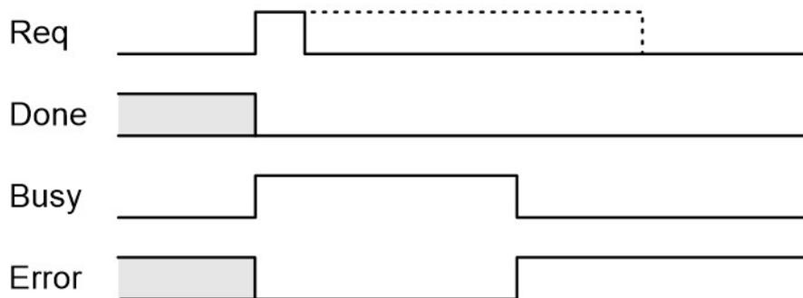
Figure 4.31 – GlobalControl DFB Timing Diagram - Failure
