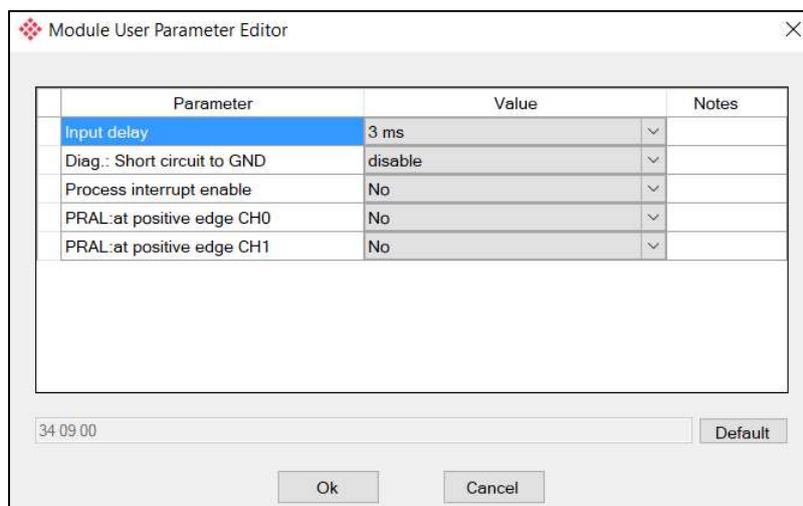
Figure 3.51 – Device Slot configuration additional parameters
