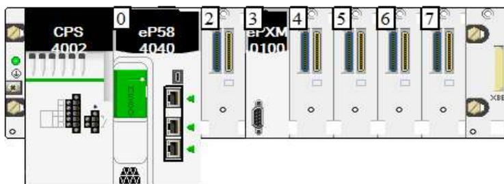
Figure 3.65 – Confirm PXM has been added to M580 backplane.
