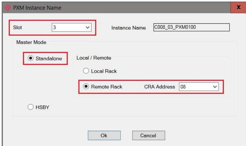
Figure 3.22 – Instance Name Builder – Standalone - Remote Rack
