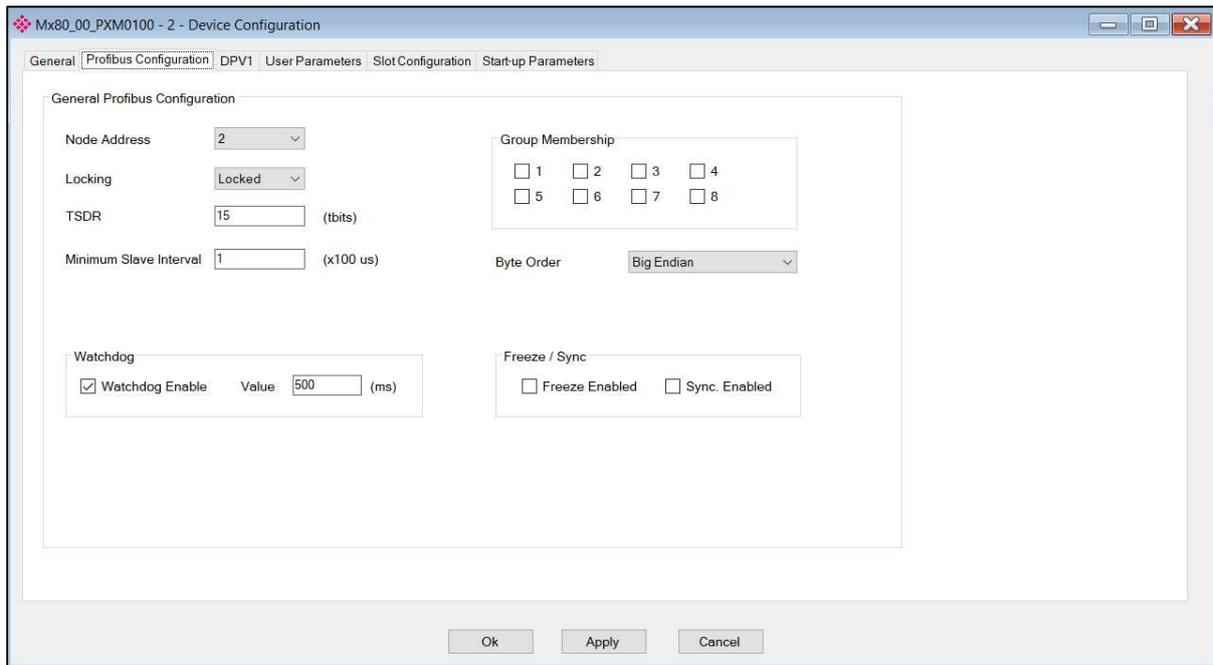
Figure 3.45 – Field Device PROFIBUS configuration parameters
