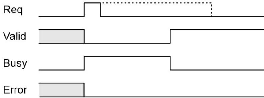
Figure 4.17 – WRRec DFB Timing Diagram - Success
