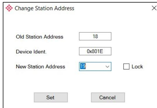
Figure 3.40 – Selecting new Station Address.
