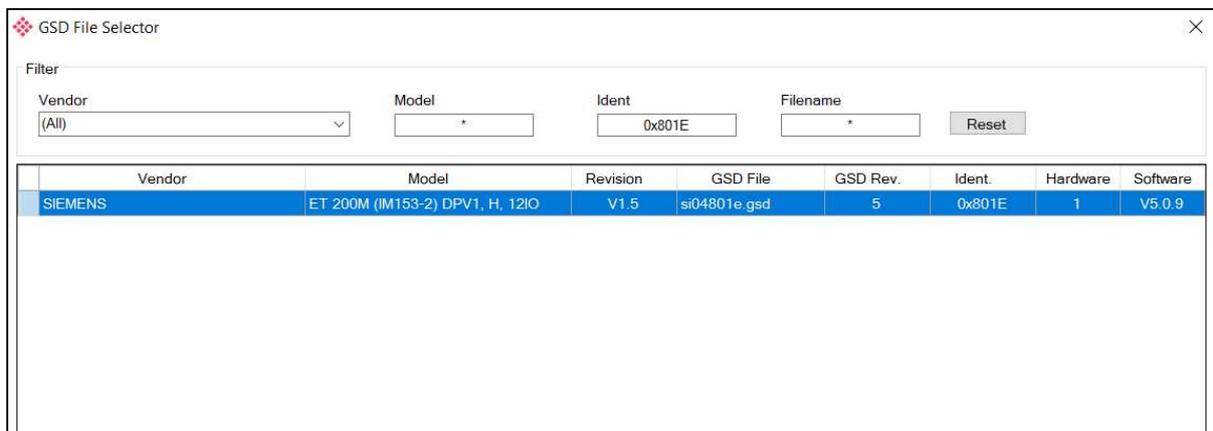
Figure 3.37 – Selecting the GSD for the slave device
