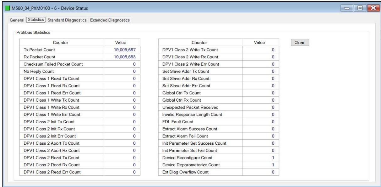
Figure 8.15 – Device Status monitoring - Statistics
