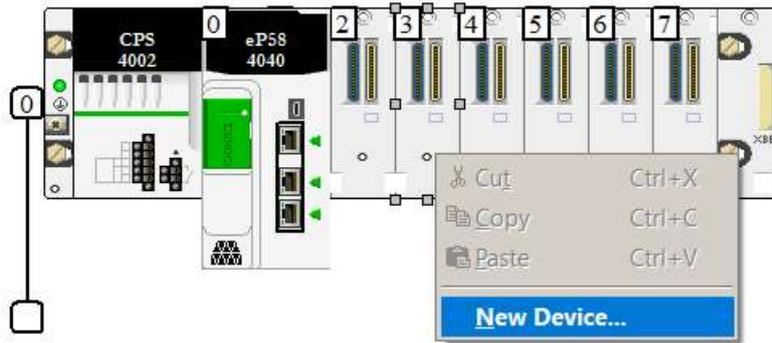
Figure 3.63 – Adding PXM in Control Expert
