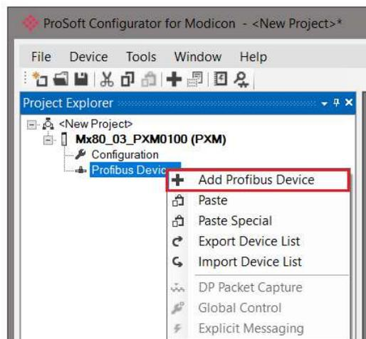
Figure 3.41 – Adding a PROFIBUS Field Device
