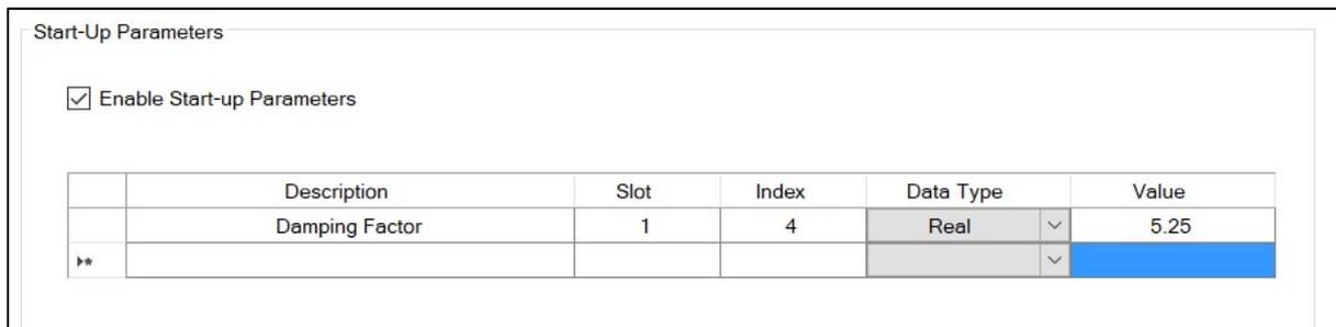
Figure 3.53 – Device Start-up Parameters Example
