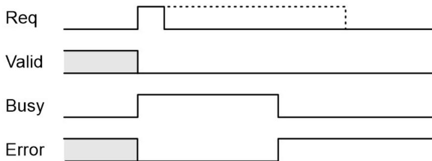
Figure 4.18 – WRRec DFB Timing Diagram - Failure
