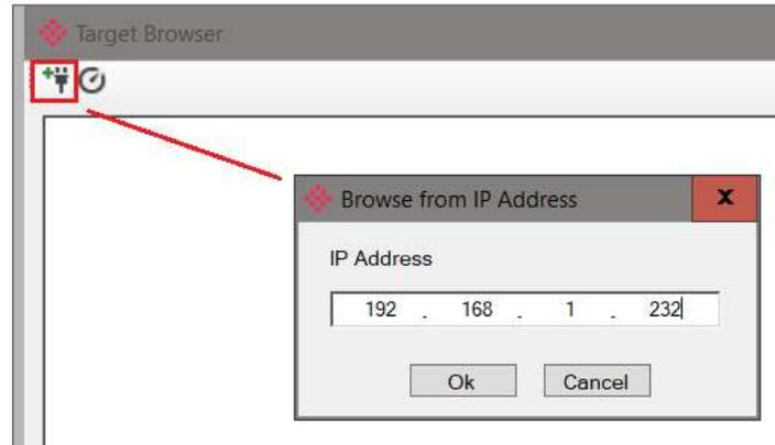
Figure 4.44 – Add PXM manually (Connecting via NOC)
