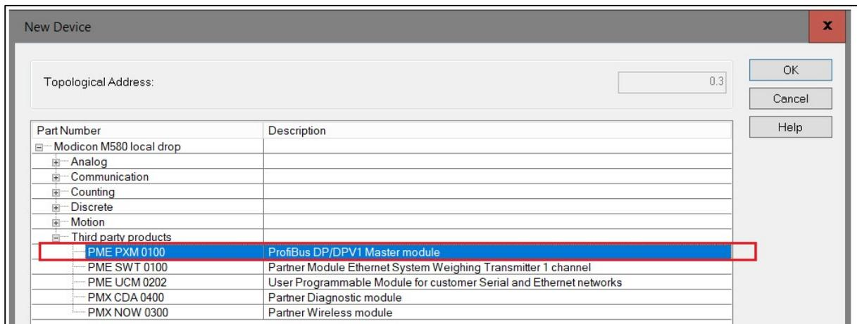
Figure 3.64 – Selecting PXM in Control Expert
