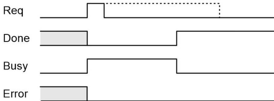
Figure 4.30 – GlobalControl DFB Timing Diagram - Success
