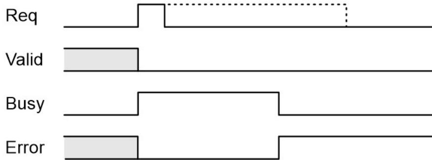
Figure 4.26 – RDAIarm DFB Timing Diagram - Failure
