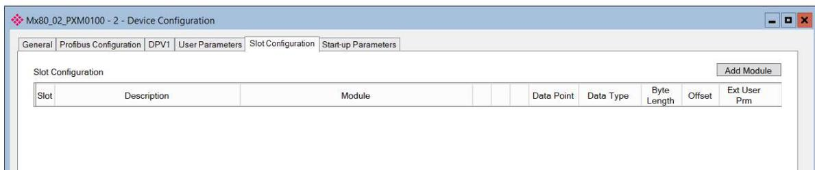
Figure 3.48 – Field Device Slot configuration start
