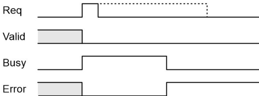
Figure 4.22 – RDDiag DFB Timing Diagram – Failure
