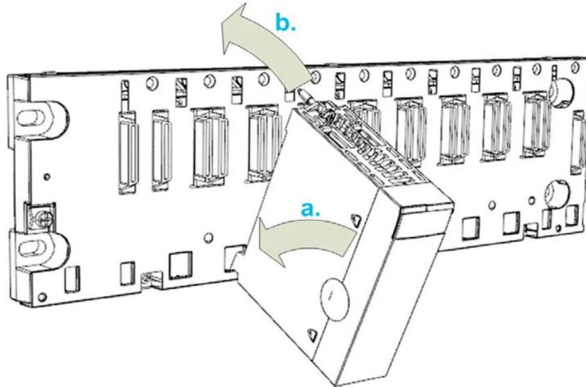
Figure 2.3 – Mounting the PXM to the backplane
