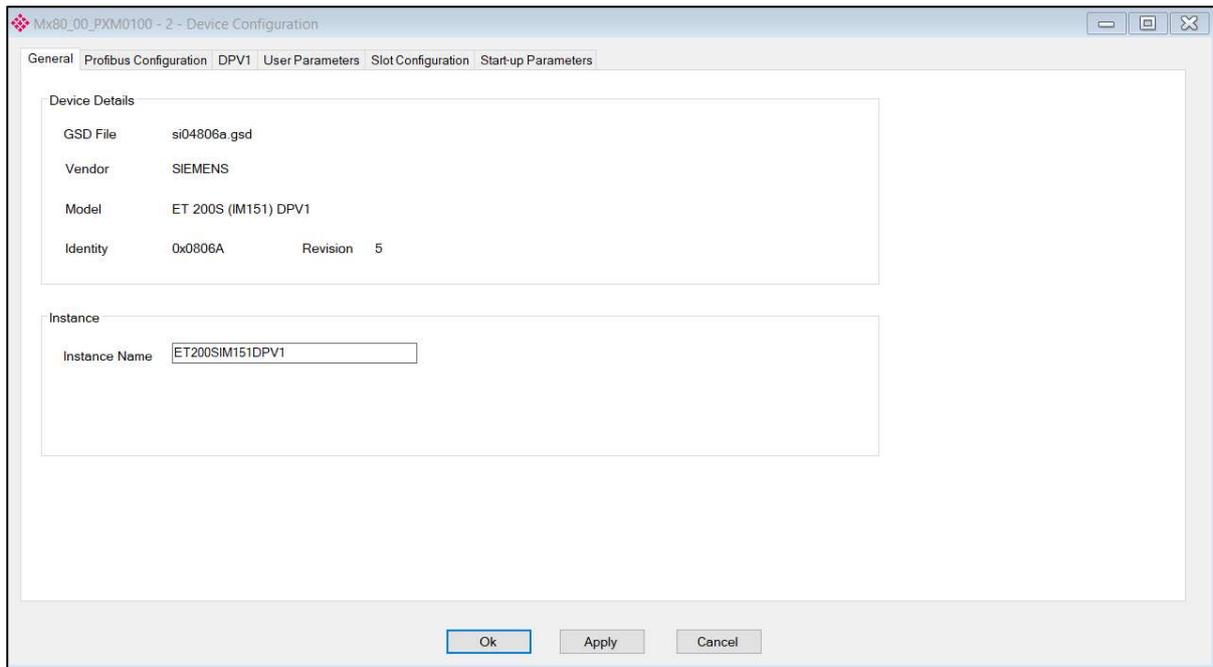
Figure 3.44 – Field Device General configuration parameters
