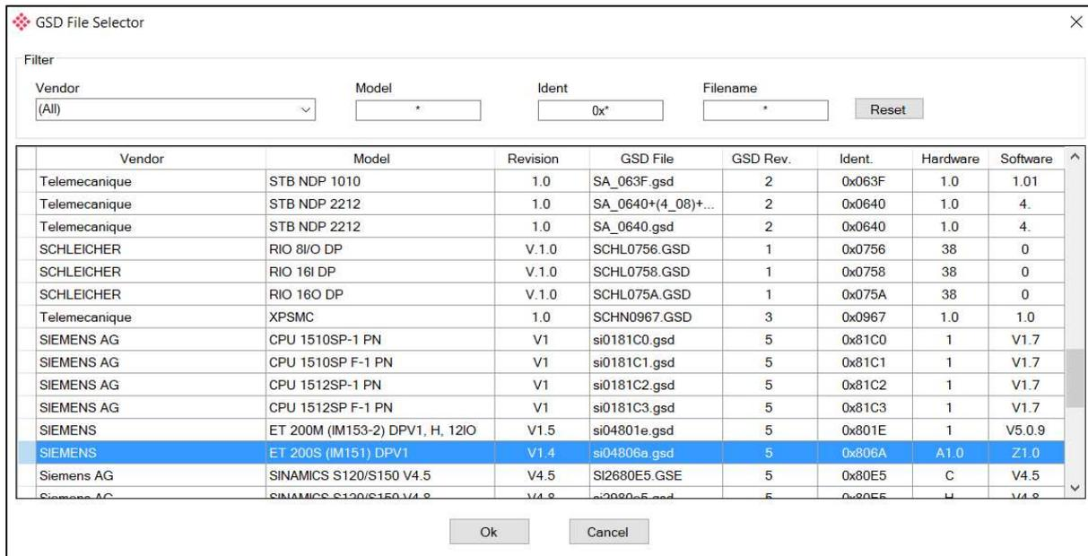
Figure 3.42 – Selecting a PROFIBUS Field Device
