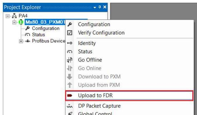
Figure 4.40 – Upload PXM Configuration to FDR
