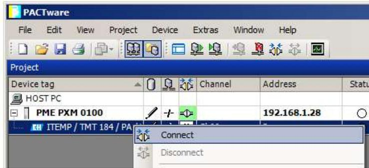
Figure 7.14 – Slave Device DTM Connect
