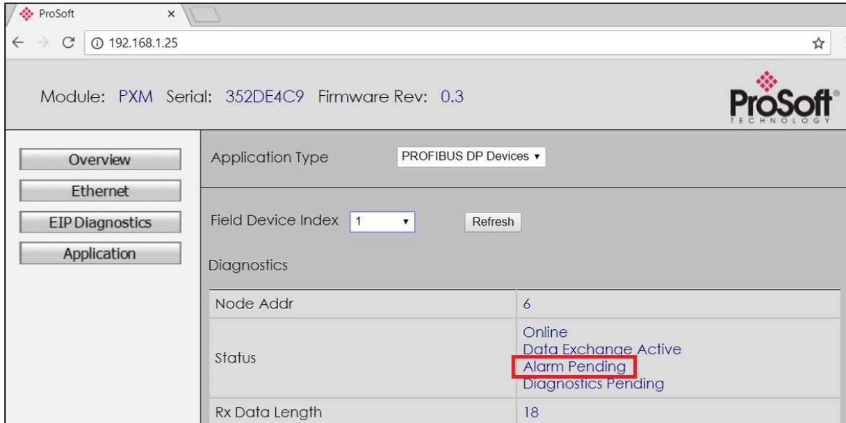
Figure 4.39 – Field device Alarm Pending in PXM Webserver
