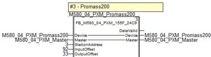
Figure 4.4 – Device Mapping DFB example
