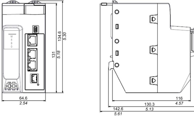
The BMEP58CPROS3 Copro presents the following physical dimensions. Unlike the CPU, the Copro does not present physical connectors or related labels
