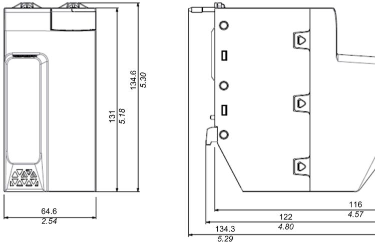
**NOTE:** Consider the height of the CPU and Copro when you are planning the installation of the local rack. Both the CPU and Copro extend below the lower edge of the rack by:
