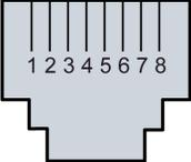
**NOTE:** The TD pins (1 and 2) and the RD pins (3 and 6) are auto-MDIX enabled and automatically reverse their roles depending on the connected media (i.e., straight or crossed cables).
