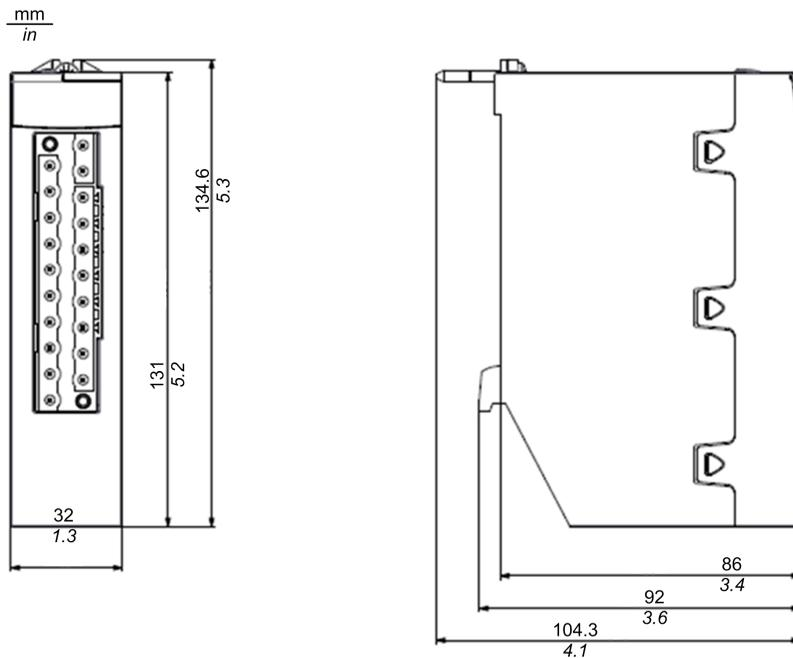
**NOTE:** Consider the height of the safety I/O modules when you are planning the installation of a rack. Each safety I/O module extends below the lower edge of the rack by:
