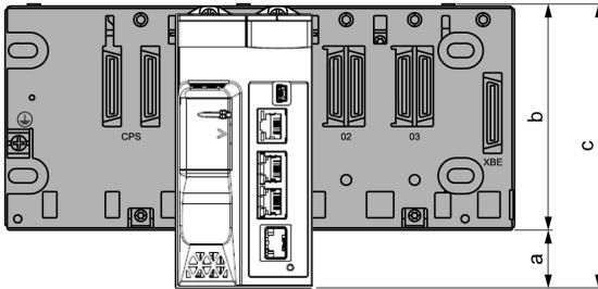
**a** Additional space below the rack to accommodate the height of the CPU. For an X Bus rack, the value is 32.0 mm (1.260 in.); for an Ethernet rack, the value is 30.59 mm (1.204 in.).
