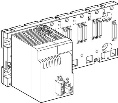
**NOTE:** The power supply module design allows it to be placed only in the dedicated slots marked **CPS**.
