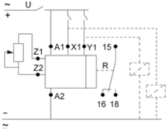
Function Ac: On-Delay & Off-Delay with Control Signal
