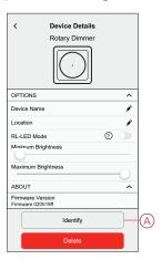
The status LED blinks red and connected lighting devices blinks On/Off, upon successful identification of the dimmer.
