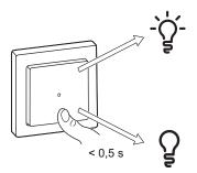
Long press the push-button (> 0,5 s) on the device to increase/decrease the brightness of the dimmer.
