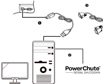
3. A built-in serial port is also available for additional communication options with serial cable.
