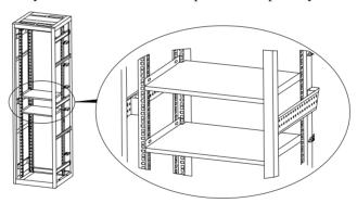
Refer to the below chart to install UPS and battery pack into 19" rack enclosure.
