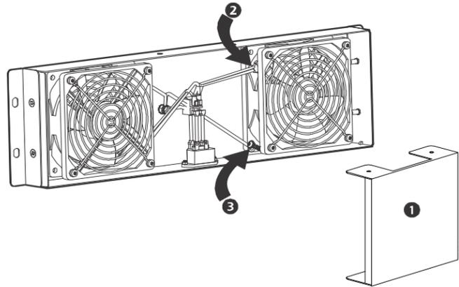
5. With a Phillips head screwdriver, remove four (4) screws from each finger guard on either side of the old fan.
