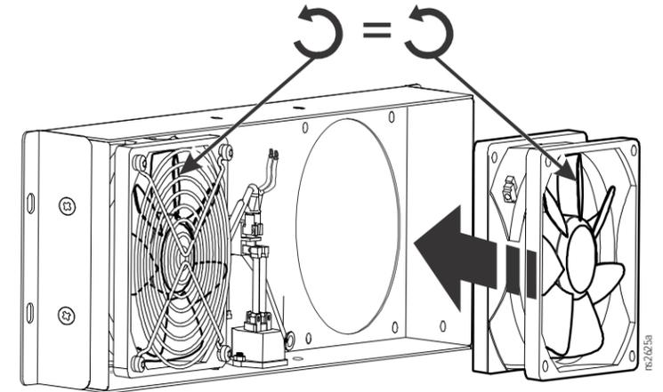
Reverse the removal steps to install the replacement fan.
