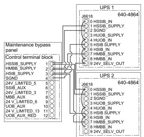
3. On UPS 2: Cut the preinstalled jumper between pins 8 and 9 on the terminal connector for J6618 on board 640-4864.
