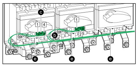
Connect the Class 2/SELV signal cables for the breaker indicator lights from the control terminal block in the maintenance bypass panel to the UPSs as per your configuration.
