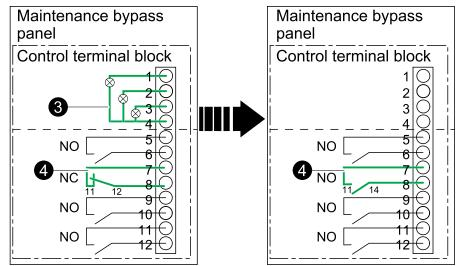
5. Connect the Class 2/SELV signal cables from the control terminal block in the maintenance bypass panel to the UPS as per your configuration.
