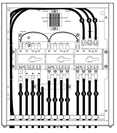
6. Fasten the cables with cable ties (provided) to the cable reliefs in the left side, top, and bottom of the maintenance bypass panel.
