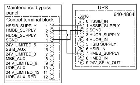
2. Connect the non-Class 2/non-SELV signal cables from the control terminal block in the maintenance bypass panel to the UPS as per your configuration.
