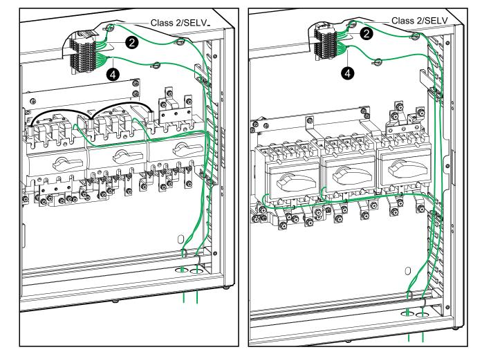
5. Pull up the slack in the signal cables and fasten the signal cables to the cable reliefs.
