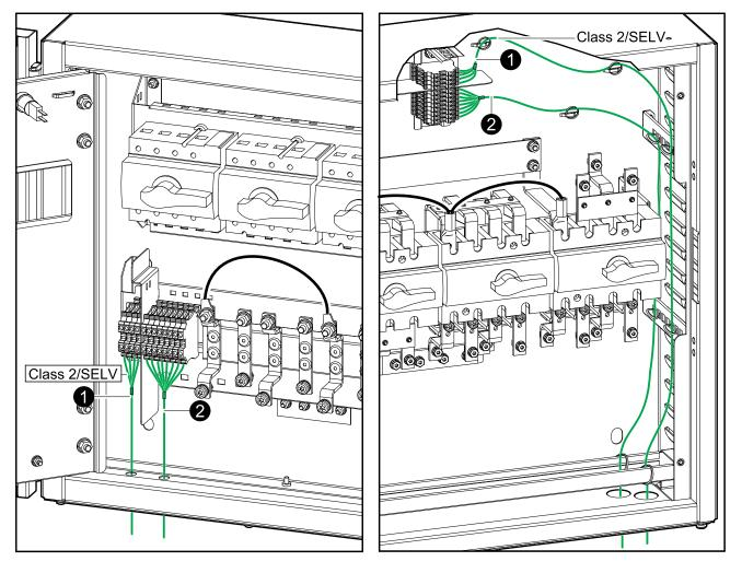
1. Connect the Class 2/SELV signal cables for the breaker indicator lights from the control terminal block in the maintenance bypass panel to the UPS as per your configuration.
