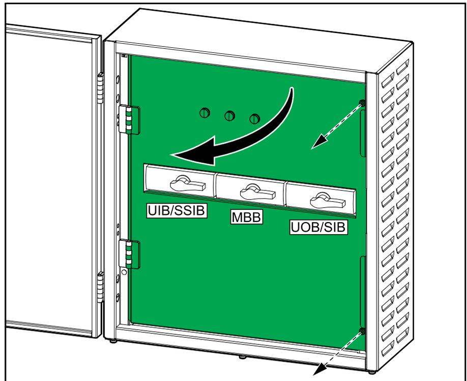
2. Measure and mark the four mounting hole locations on the wall.
