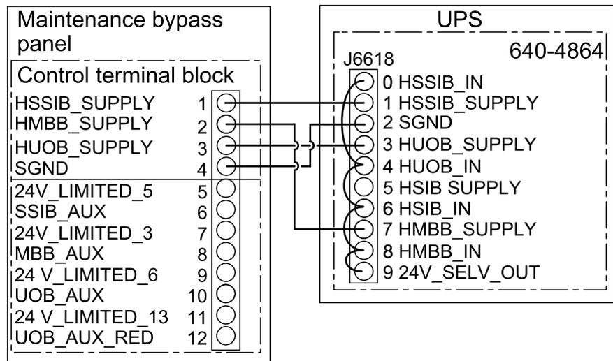
2. Connect the non-Class 2/non-SELV signal cables from the control terminal block in the maintenance bypass panel to the UPS as per your configuration.
