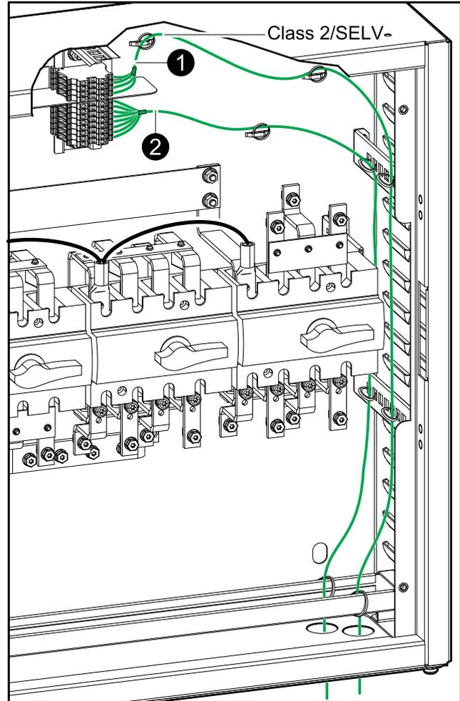
1. Connect the Class 2/SELV signal cables for the breaker indicator lights from the control terminal block in the maintenance bypass panel to the UPS as per your configuration.
