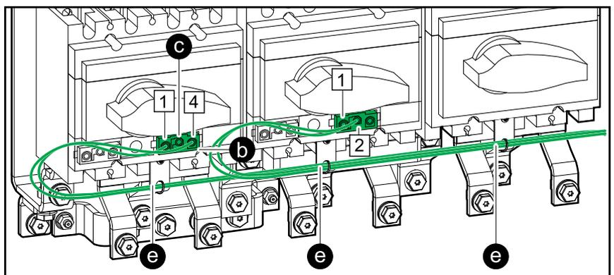
2. Connect the Class 2/SELV signal cables for the breaker indicator lights from the control terminal block in the maintenance bypass panel to the UPSs as per your configuration.
