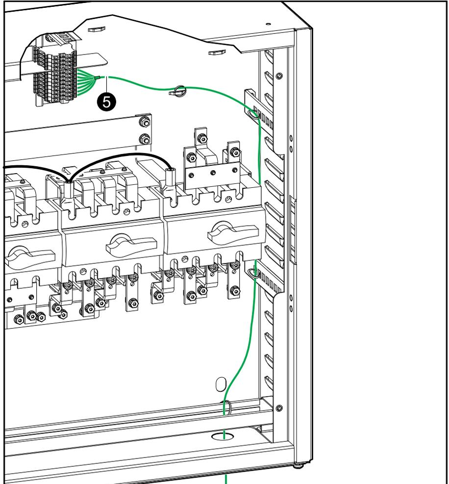
**NOTE:** There is no dedicated input contact on Easy UPS 3S for MBB. By default use J5 configurable input contact, configure as **Main CB NO.**
