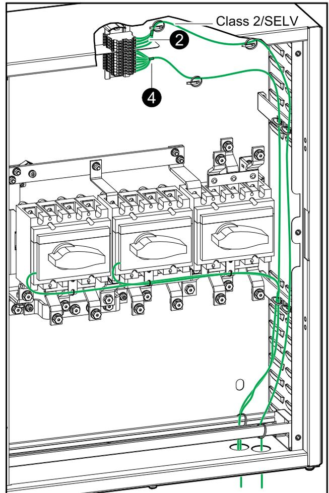
5. Pull up the slack in the signal cables and fasten the signal cables to the cable reliefs.
