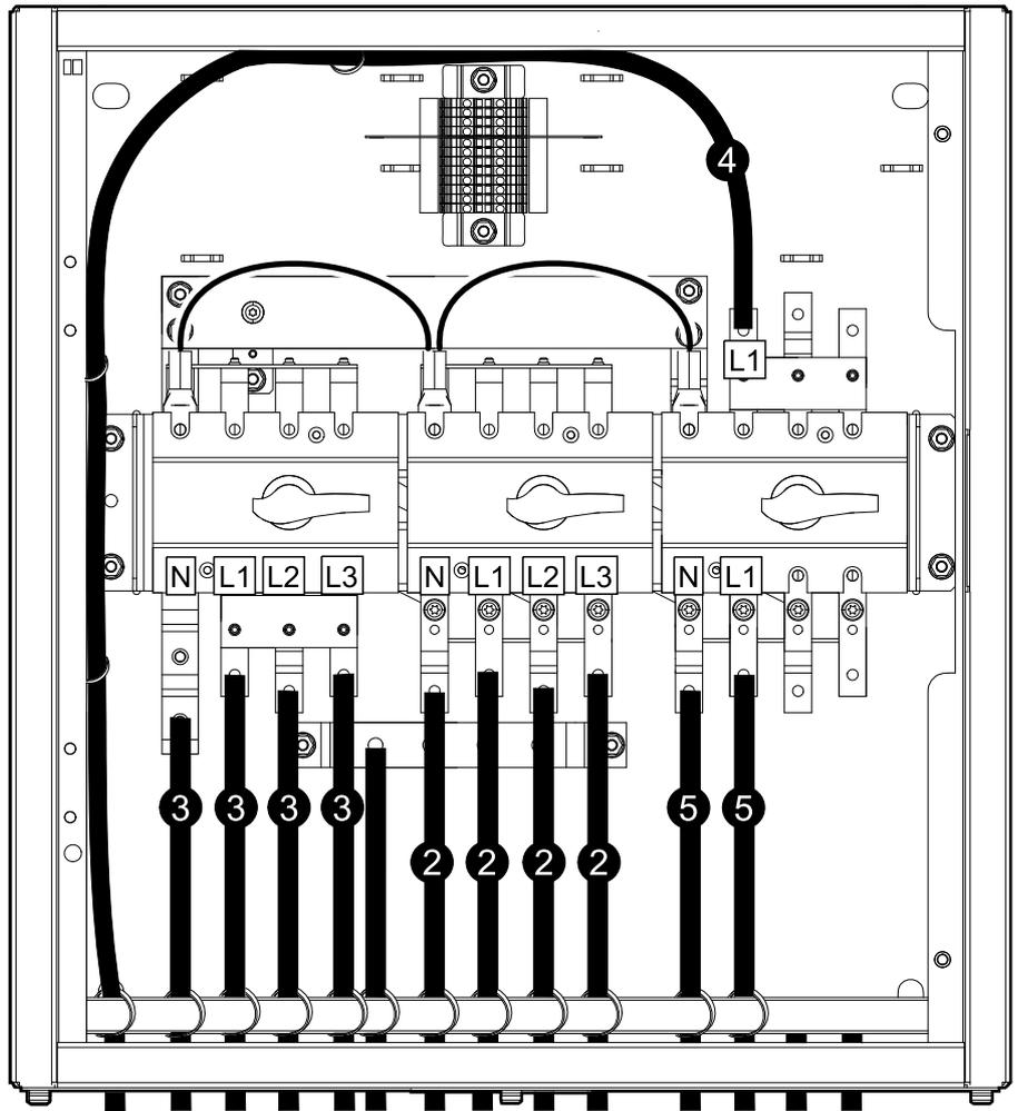
6. Fasten the cables with cable ties (provided) to the cable reliefs in the left side, top, and bottom of the maintenance bypass panel.
