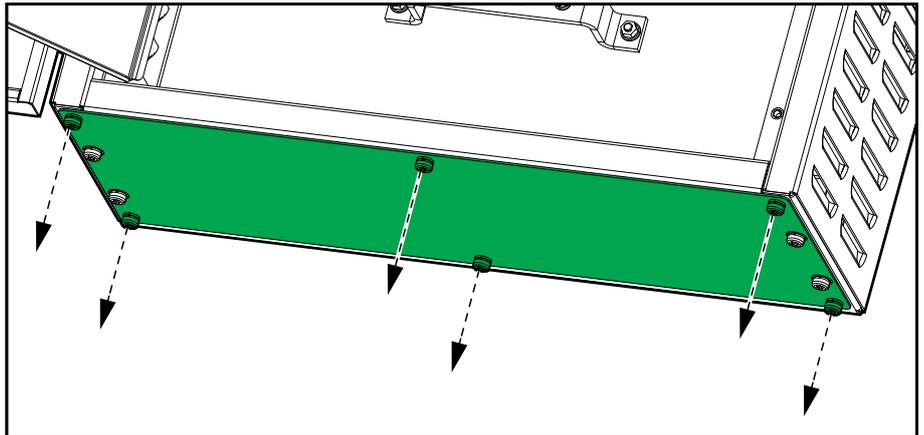
2. Drill or punch holes for cables or grommets in the gland plate.
