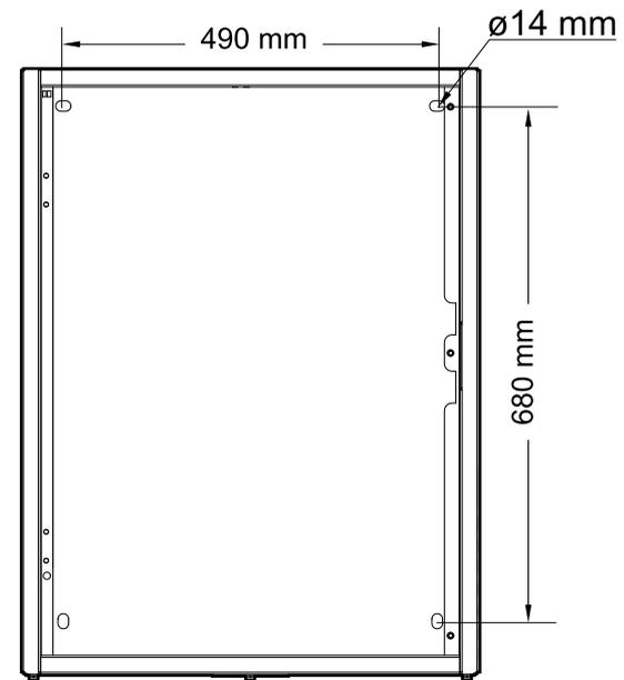
3. Drill holes in the four marked locations and mount the anchor bolts.
