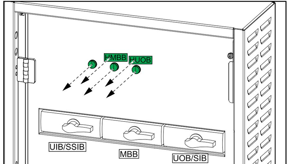
2. Install three round blanking plugs (not provided) in the holes in the inner door.
