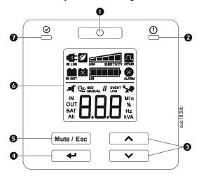
• Press the DOWER ON/OFE button to turn the LIPS on
