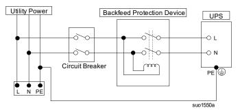
Use external backfeed protection device as per the table below.
