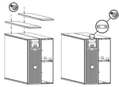
2. Install the tie bracket securing the UPS and external battery pack (screws included).
