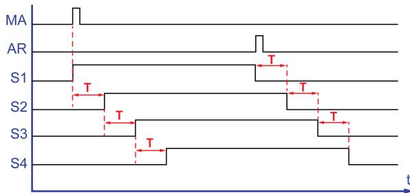
An On (**MA**) button authorizes the activation of the first heating element (**S1**). After a time-delay  $T$ , the second element (**S2**) starts up. After the same time-delay, the third elements starts up (**S3**), then the fourth element (**S4**) again after time-delay  $T$ . An Off (**SR**) button deactivates (**S1**). The three other elements are progressively deactivated after time-delay  $T$ .
