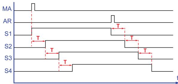
An On (**MA**) button authorizes the activation of the first heating element (**S1**). After a time delay **T**, the second element (**S2**) starts up. After the same time delay, the third element starts up (**S3**), then the fourth element (**S4**) again after time-delay **T**. An Off (**AR**) button deactivates **S1**. The three other elements are progressively deactivated after time delay **T**.
