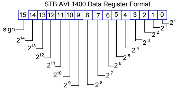
All 16 bits in each data word are significant. They allow you to represent analog input voltages with all the integer values ranging from -32 768 to 32 767.
