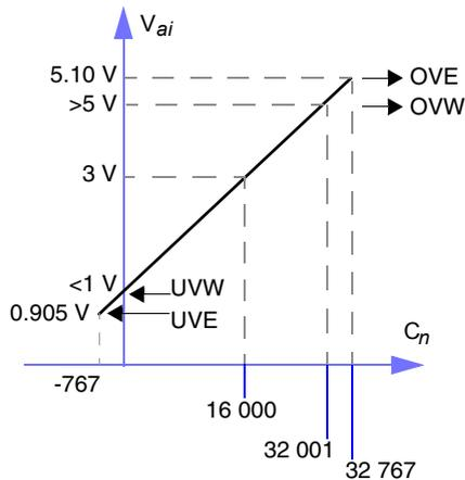
In an ideal linear voltage representation for 0 to 5 VDC range (one with default offset or max count settings (see *p. 228*)), a value of 32 001 represents an OVW. If the input value is less than or equal to 767, the module will report a UVW. When the input value reaches 32 767, an OVE occurs. When the input value reaches 0, a UVE occurs.
