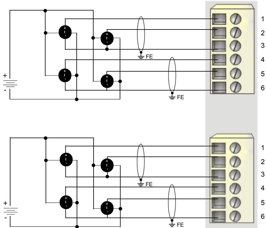
Notice that the return lines for the sensors are connected in external junction boxes so that two returns are brought into pins 3 and 6 on both connectors with a single wire.
