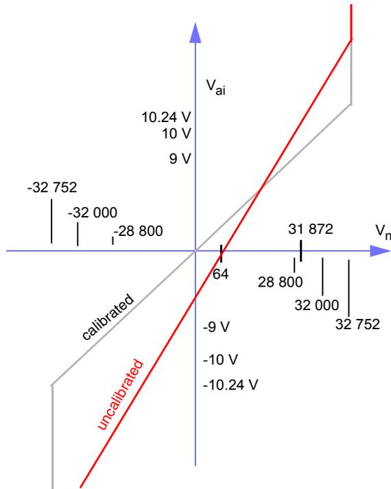
Here are some voltage representations after calibration with offset and max count:
