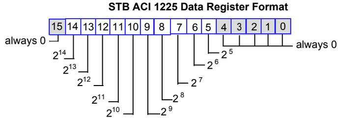
There are 10 significant bits in each data word—bits 14 through 5. They allow you to represent current data with integer values ranging from 0 to 32,736 in increments of 32. A value 32 000 represents an input of 20 mA. A value of 0 represents an input less than or equal to 4 mA.
