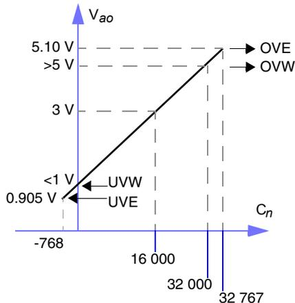
In an ideal linear voltage representation for 0 to 5 VDC range, a value of 32 001 represents an OVW. If the output value is less than or equal to 767, the module reports a UVW. When the output value reaches 32 767, an OVE occurs. When the output value reaches 0, a UVE occurs.
