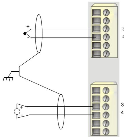
**top connector** thermocouple sensor
