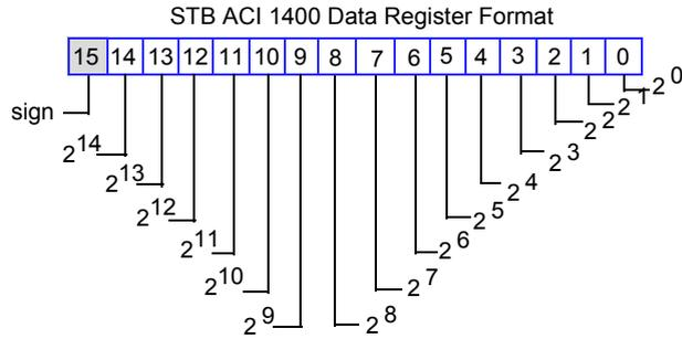
All 16 bits in the register are significant. They allow you to represent analog input currents with all the integer values in the range -32 768 to +32 767.
