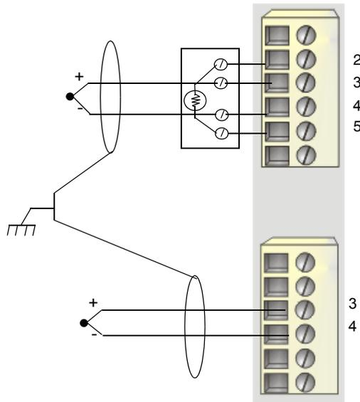
Cold-junction compensation is configured at the module level, and therefore it applies to any TC sensor(s) connected to the top and/or bottom connector on the STB ART 0200 module.
