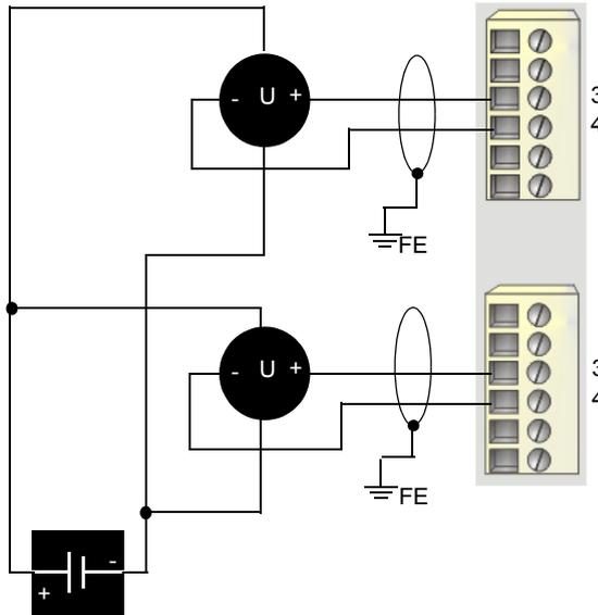
The following field wiring example shows how two wire isolated analog actuators can be wired to the STB AVO 0200 module. An external power supply is required for each channel:
