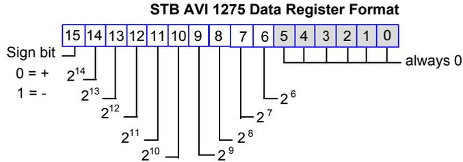
There are 10 significant bits in each data word—bits 15 through 6. They allow you to represent voltage data with integer values ranging from -32 768 to +32 704 in increments of 64. A value 32 000 represents +10 V and a value of -32 000 represents -10 V. When bit 15 is 0, the value is positive; when bit 15 is 1, the value is negative.
