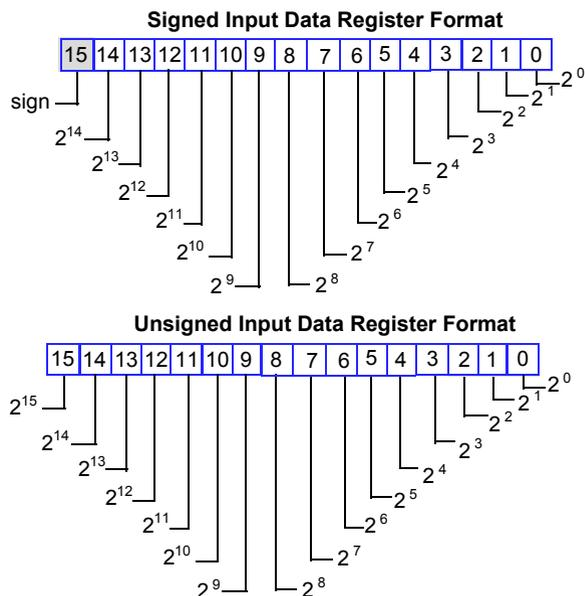
Each data word allows you to represent analog input current data with either signed integer values ranging from -32 767 to 32 767 or with unsigned integer values in the range 0 to 65 534.
