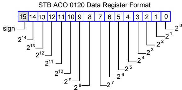
All 16 bits in the data word are significant. They allow you to represent analog output current data with all the integer values in the range -1 000 to 32 767.
