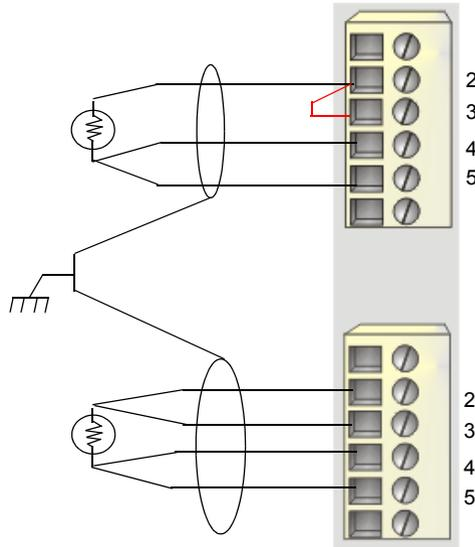
Double-shielded cable may be used with two-, three- or four-wire RTDs operating in high-noise environments. The example below shows a two-wire RTD set-up with double-shielded, twisted-pair cable:
