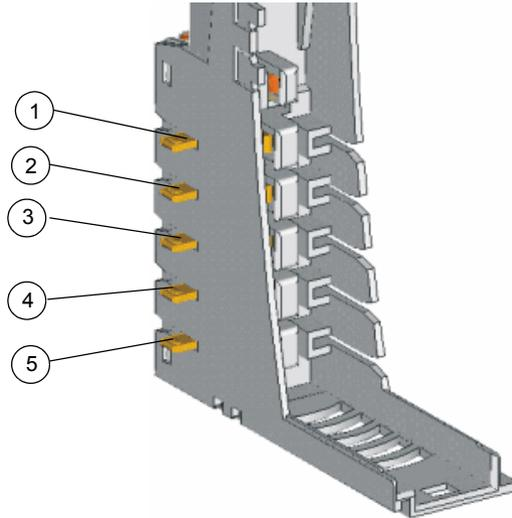
Field power (sensor power for inputs and actuator power for outputs) is distributed across the island bus to the STB XBA 1000 bases by a PDM:
