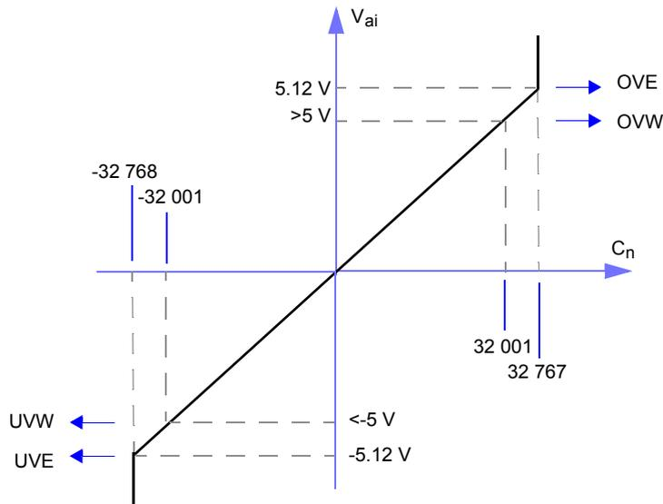
In an ideal linear voltage representation for +/-10 VDC range (one with default offset or max count settings (see *p. 228*)), a value of 32 001 represents an OVW. If the input value is less than or equal to -32 001, the module will report a UVW. When the input value reaches 32 767, an OVE occurs. When the input value reaches -32 767, a UVE occurs.
