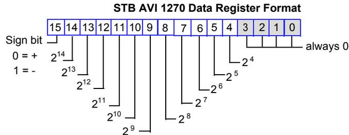
There are 12 significant bits in each data word—bits 15 through 4. They allow you to represent voltage data with integer values ranging from -32 768 to +32 752 in increments of 16. When the sign bit (bit 15) is 0, the value is positive; when bit 15 is 1, the value is negative.
