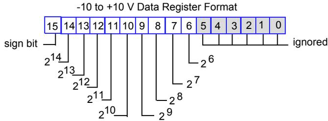
The value of each data word is represented in bits 15 through 6, The bits represent voltage data as integer values in the range -32 768 ... +32 704 in increments of 64. When the sign bit (bit 15) is 0, the value is positive; when bit 15 is 1, the value is negative.
