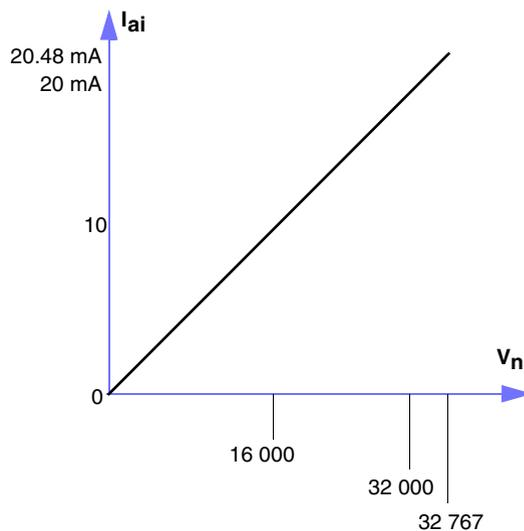
For example, if you use the Advantys configuration software to calibrate an offset of +64 at 4 mA and a max count of 31 744 at 20 mA, the system could be represented as follows:
