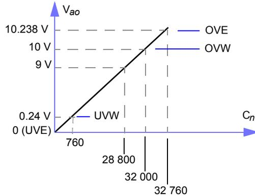
When the voltage range is from -10 to +10 VDC, voltage data is represented as follows:
