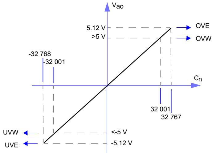
In an ideal linear voltage representation for  $\pm 10\text{ VDC}$  range, a value of 32 001 represents an OVW. If the output value is less than or equal to -32 001, the module reports a UVW. When the output value reaches 32 767, an OVE occurs. When the output value reaches -32 768, a UVE occurs.
