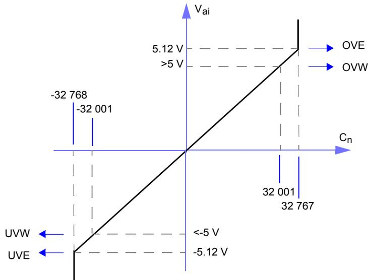
In an ideal linear voltage representation for +/-10 VDC range (one with default offset or max count settings (see *p. 203*)), a value of 32 001 represents an OVW. If the input value is less than or equal to -32 001, the module reports a UVW. When the input value reaches 32 767, an OVE occurs. When the input value reaches -32 768, a UVE occurs.
