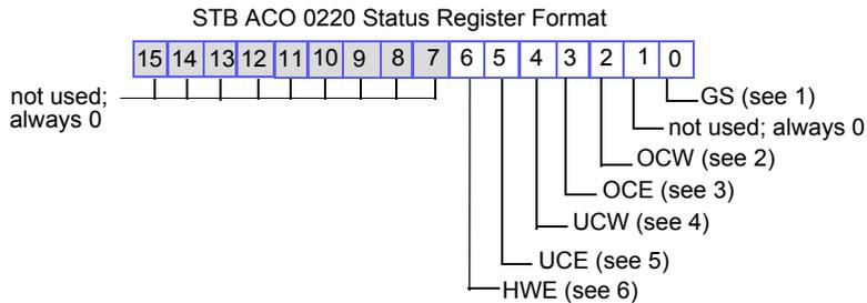
1. Bit 0 represents global status (GS). It has a value of 0 when no errors have been detected. It has a value of 1 when bit 6 has a value of 1.
