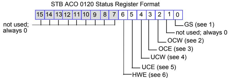
1. Bit 0 represents global status (GS). It has a value of 0 when no errors are detected. It has a value of 1 when bit 6 has a value of 1.
