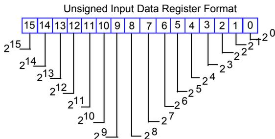
Each data word allows you to represent analog output current data with either signed integer values ranging from -32 767 to 32 767 or with unsigned integer values in the range 0 to 65 534.
