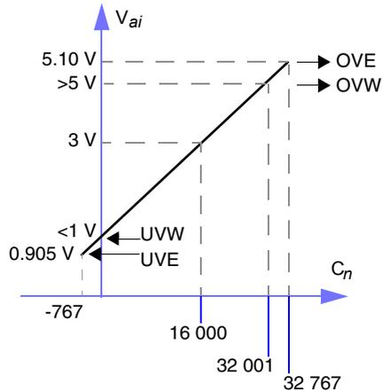
In an ideal linear voltage representation for 0 to 5 VDC range (one with default offset or max count settings (see *p. 203*)), a value of 32 001 represents an OVW. If the input value is less than or equal to 767, the module reports a UVW. When the input value reaches 32 767, an OVE occurs. When the input value reaches 0, a UVE occurs.
