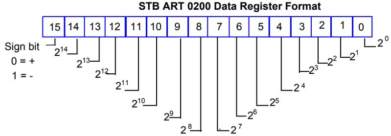
If a register holds temperature data, it represents it as degree C x 10 or degrees F x 10. For example, if the channel data is 74.9 degrees C, the register representing that channel reads 749 (in decimal) or 0x2ED (in hexadecimal). You can configure degree C or degrees F in the module editor (see p. 160).
