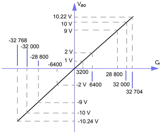
Values greater than 32 000 and less than -32 000 do not produce out-of-range indications.
