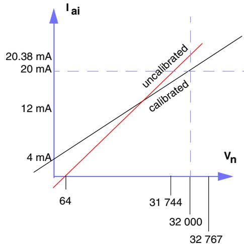
Here are some current representations after calibration with offset and max count:
