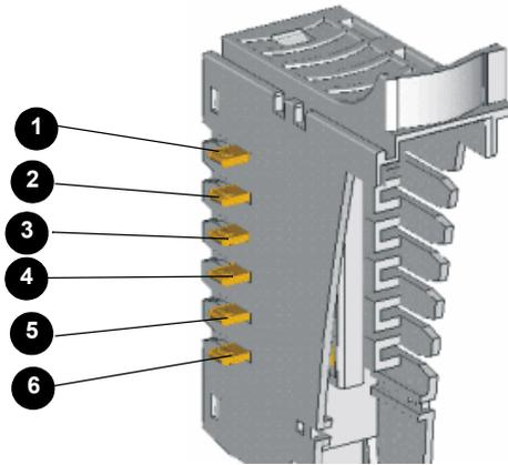
In the primary segment of the island bus, the signals that make these contacts come from the NIM. In extension segments, these signals come from an STB XBE 1000 BOS extension module:
