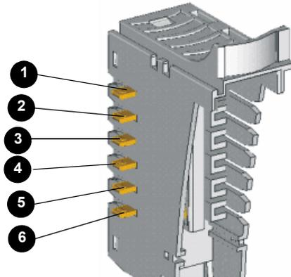
In the primary segment of the island bus, the signals that make these contacts come from the NIM. In extension segments, these signals come from an STB XBE 1000 BOS extension module:
