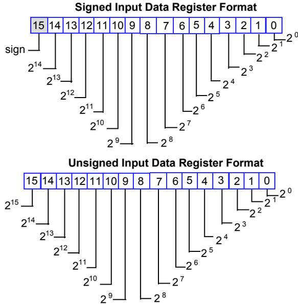
Each data word allows you to represent analog input current data with either signed integer values ranging from -767 to 32 767 or with unsigned integer values in the range 0 to 65 535.
