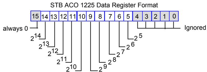
The value of each data word is represented in bits 14 through 5. The bits represent current data as integer values in the range 0 to 32,736 in increments of 32. A value 32 000 results in a 20 mA output, and a value of 0 results in a 4 mA output.
