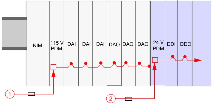
Each basic PDM contains on 5 A time-lag fuse that protects the I/O modules in the segment. This fuse is user-replaceable.
