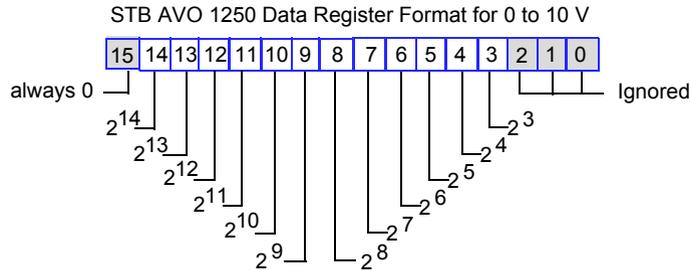
In this case, you can represent voltage data with integer values in the range 0... +32 760 in increments of 8. The value of bit 15 should always be 0. If a negative value is sent, the output will be set to 0 VDC and an under-voltage error will be returned. The value 32 000 produces a 10 V output, and the value 0 produces a 0 V output. If the output value is set to 32 760 or greater, an over-voltage error (OVE) is reported.
