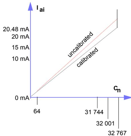
Here are some current representations after calibration with offset and max count:
