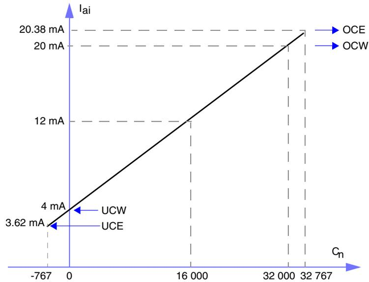
In the 0 to 20 mA operating range, an ideal linear representation of analog input current (one with default offset and maximum count) is given by the following formula:
