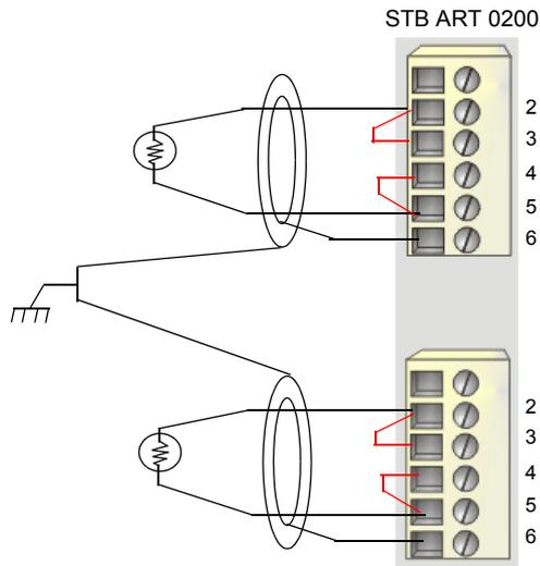
When double-shielded twisted-pair cable is used, the inner shield is tied to pin 6. Pin 6 is not used when standard (single-shielded) twisted-pair cable is used.
