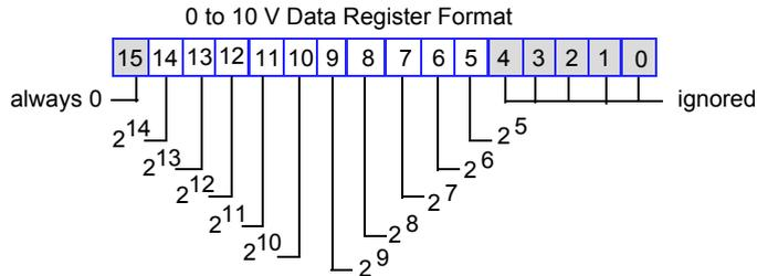
There are 10 significant bits in each data word—bits 14 through 5. They allow you to represent voltage data with integer values ranging from 0 to 32,736 in increments of 32. A value 32 000 results in an output of 10 V. If the sign bit (bit 15) is set, the output is set to 0 V.
