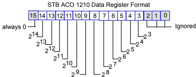
There are 12 significant bits in each data word—bits 14 through 3. They allow you to represent current data with integer values ranging from 0 to 32,760 in increments of eight.
