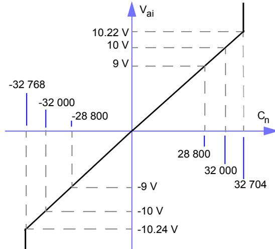
Values greater than 32 000 and less than -32 000 do not produce out-of-range indications.
