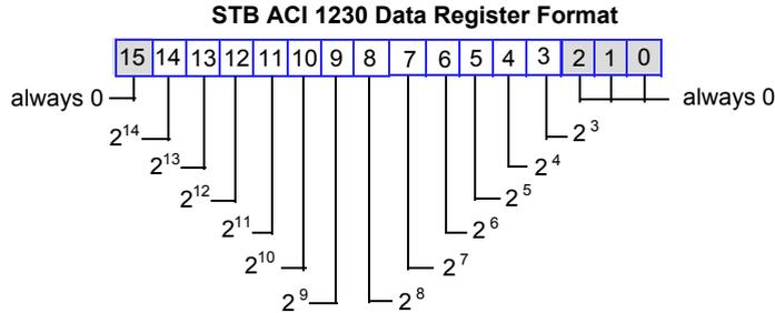
There are 12 significant bits in each data word—bits 14 through 3. They allow you to represent current data with integer values ranging from 0 to 32,760 in increments of eight.
