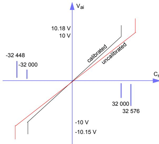
Here are some voltage representations after calibration with offset and max count:
