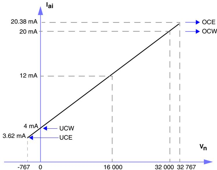
**In the 0 to 20 mA operating range**, linear current representations can be interpreted using the formula, where  $V_n$  is the numerical count and  $I_{ai}$  is the analog input current:
