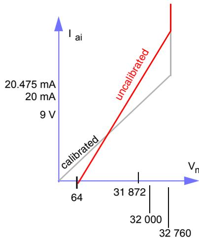
Here are some current representations after calibration with offset and max count:
