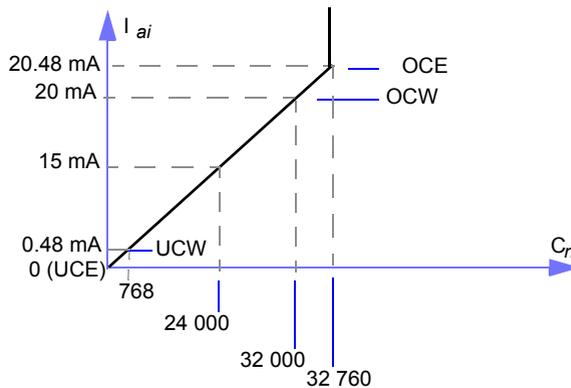
The sign bit (bit 15) is always 0, indicating that negative values are not represented. The three least significant bits in the data words are always 0.
