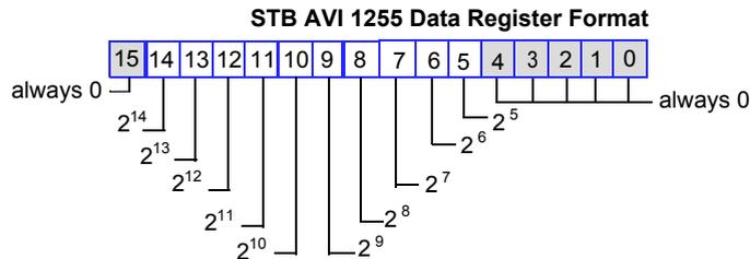
There are 10 significant bits in each data word—bits 14 through 5. They allow you to represent voltage data with integer values ranging from 0 to +32 736 in increments of 32. A value 32 000 represents an input of 10 V.
