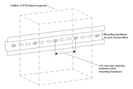
Low profile (7.5 mm deep) DIN mounting rail may be used with low profile mounting hardware such as flat head screws, with countersunk mounting holes.
