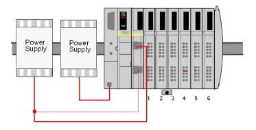
Here is a 24 V parallel power scheme for an Advantys STB island with a standard PDM:
