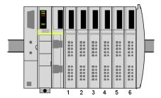
Suppose you have an STB DDO 3230 output module in address location 4, and it is malfunctioning. When you remove the module from its base, as shown below, the remaining five I/O modules in locations 1, 2, 3, 5 and 6 will continue to operate.
