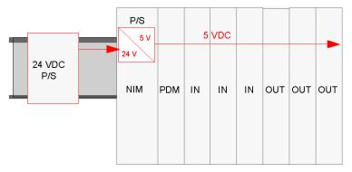
The maximum current draw from the I/O modules is limited to 1.2 A. If you place more I/O modules in the primary segment than the NIM's power supply can support (requiring more than 1.2 A of current), you may install an STB CPS 2111 auxiliary power supply to provide logic power to the additional I/O modules.
