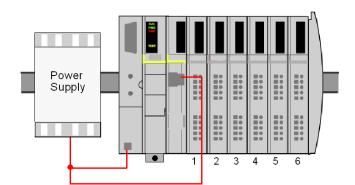
Here is a 24 V parallel power scheme for an Advantys STB island with a basic PDM:
