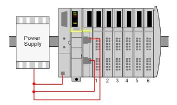
Here is an independent power scheme for an Advantys STB island with a basic PDM using two power supplies:
