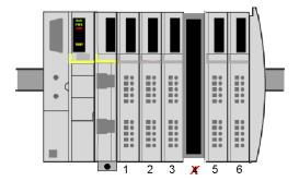
and then the RST button on the NIM is pushed, the modules in locations 1, 2 and 3 will remain operational, and the modules to the right of the empty location will not be detected.
