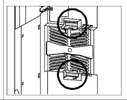
5 When the module is pushed completely on to the rail, the clips will snap closed.
