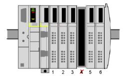
If you then place a new STB DDO 3230 output module in location 4, the NIM will recognize its device profile, configure it like the old module, and start supporting all six I/O modules the same as it did before the hot swap.
