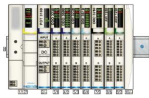
After you assign Virtual Placeholder status to the DRC 3210 digital relay output module (by selecting **Not Present** in its Options tab), the Advantys STB configuration software marks the virtual placeholder module with a red "X" as shown below:
