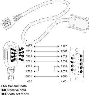
RXD receive data DSR data set ready DTR data terminal ready RTS request to send CTS clear to send GND ground reference N/C not connected
