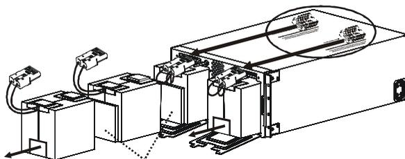
Pull the battery disconnect cords attached to the battery connectors. **DO NOT** pull the battery cables to disconnect the batteries.
