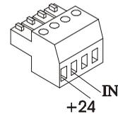
**The EPO interface is a Safety Extra Low Voltage (SELV) circuit. Connect it only to other SELV circuits. The EPO interface monitors circuits that have no determined voltage potential. Such closure circuits may be provided by a switch or relay properly isolated from the utility. To avoid damage to the UPS, do not connect the EPO interface to any circuit other than a closure type circuit.**
