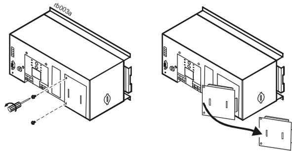
2 Remove the knockout panel that will be most convenient for connecting the external battery. Use a screwdriver to remove the knockout panel.
