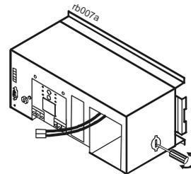
3 Locate the external battery cable and the strain relief included in the box with the battery. Clamp the strain relief on to the external battery cable. **NOTE: Once the strain relief has been clamped around the cable it can not be opened nor removed from the cable.** Slide the external battery cable through the hole in the UPS. Snap the strain relief into the hole in the UPS.
