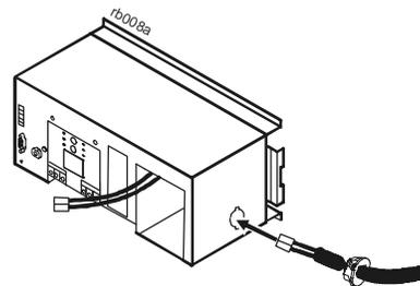
4 Firmly push the two battery connectors together. Place the battery connectors into the battery compartment.
