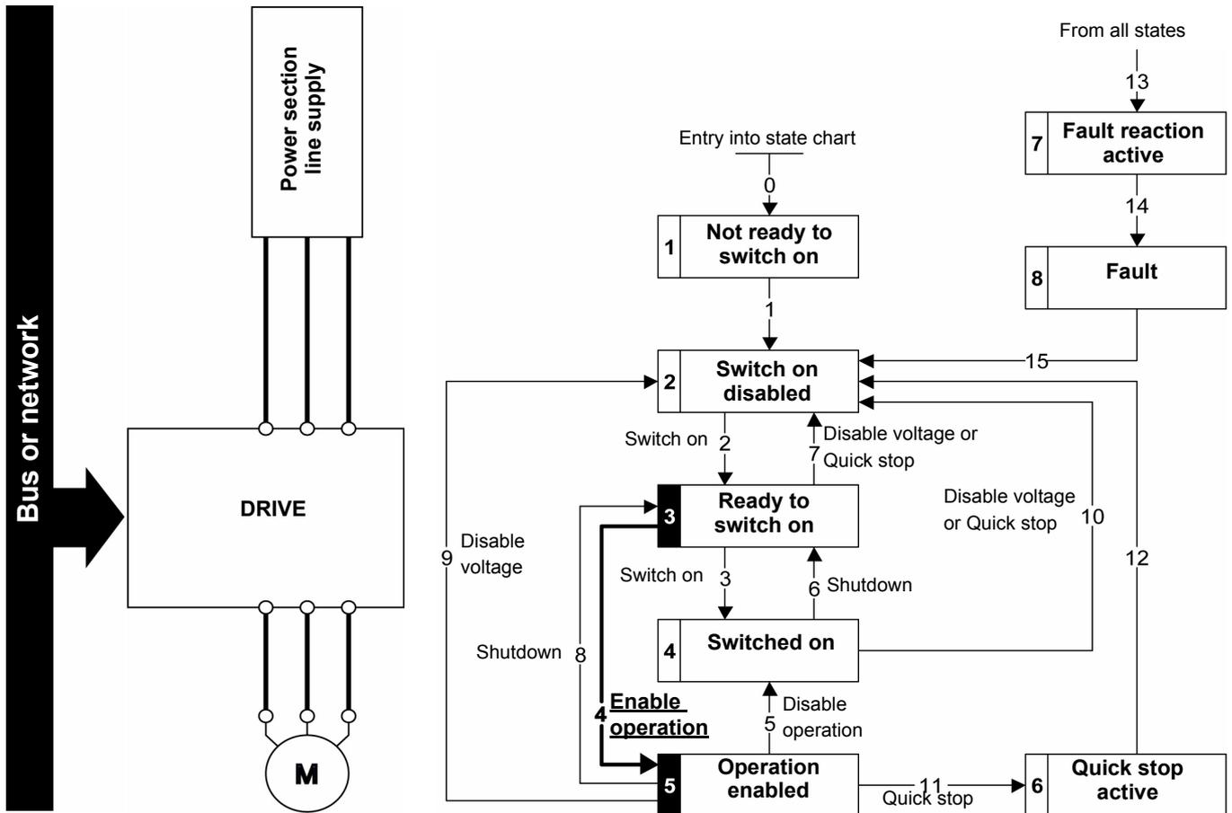
**NOTE:** It is possible, but not necessary, to send the "3 - Switch on" command followed by the "4 - Enable Operation" command to switch successively into the states "3 - Ready to Switch on", "4 - Switched on" and then "5 - Operation Enabled".
