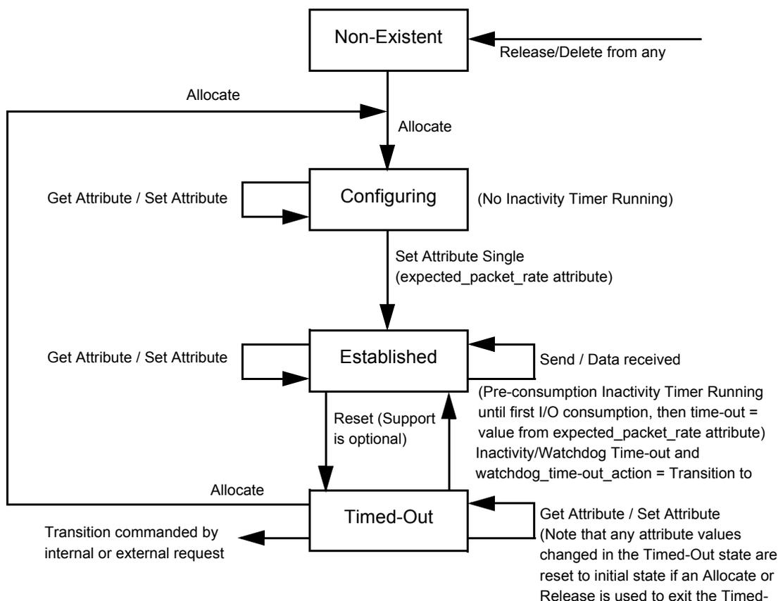
**NOTE:** The Allocate and Release services send the connection instance back to initial state. All Object attributes are reset to their default values.
