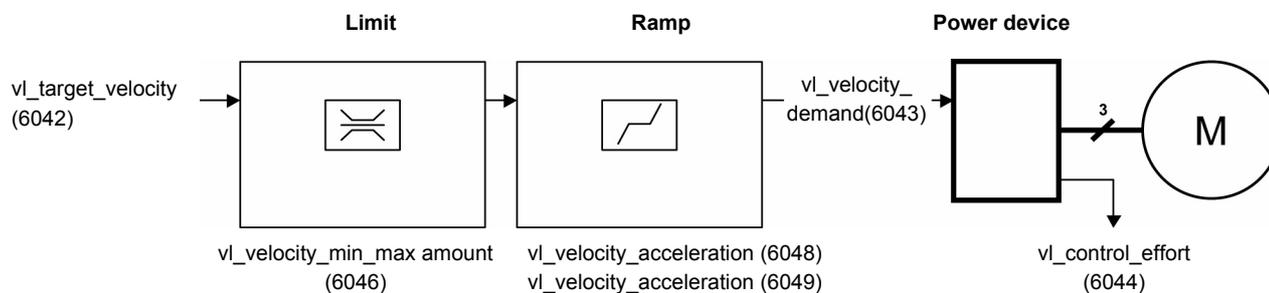
The main parameters are shown with their CiA402 name and their CiA402/Drivecom index (the values in brackets are the parameter codes).
