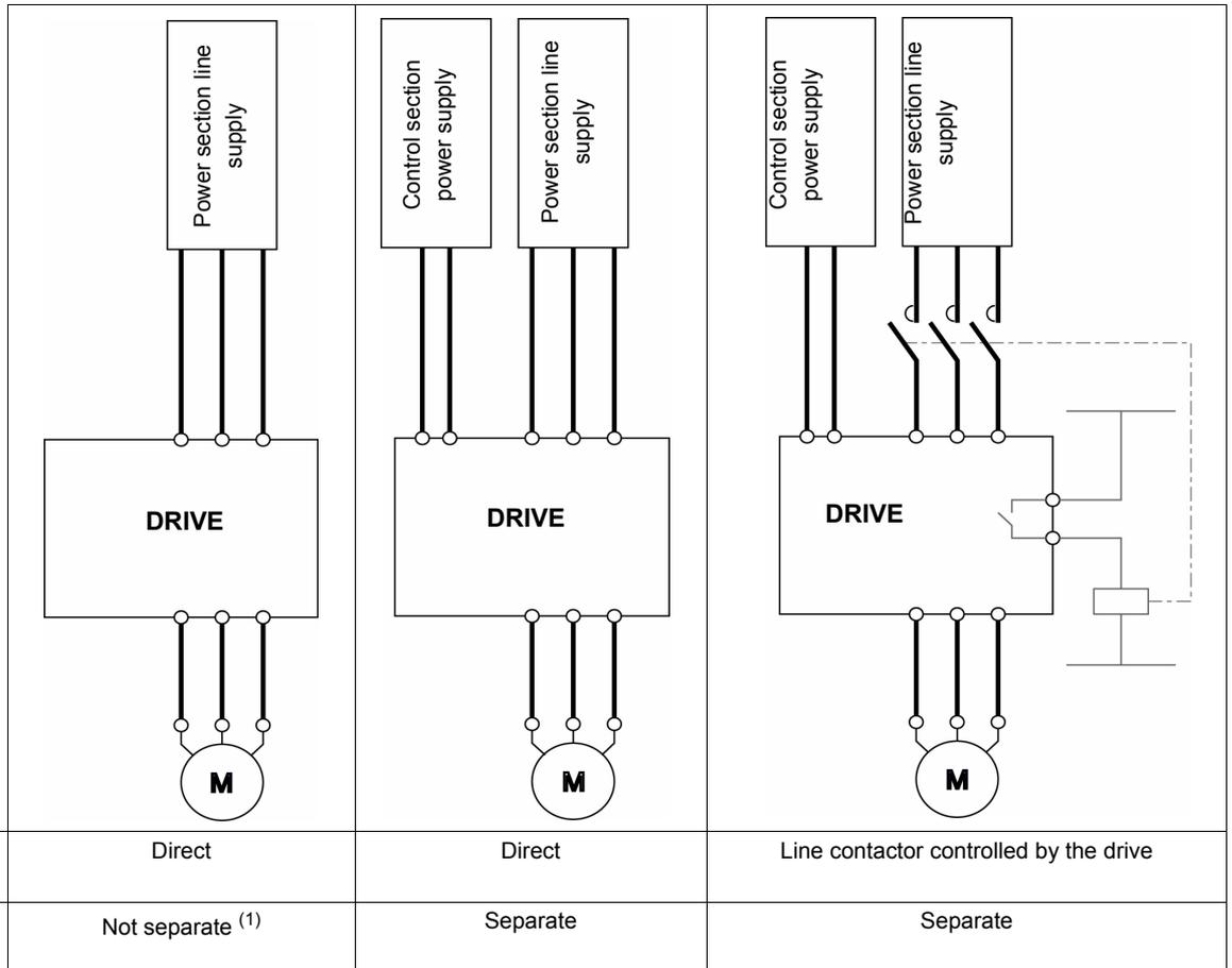
(1) The power section supplies the control section.
