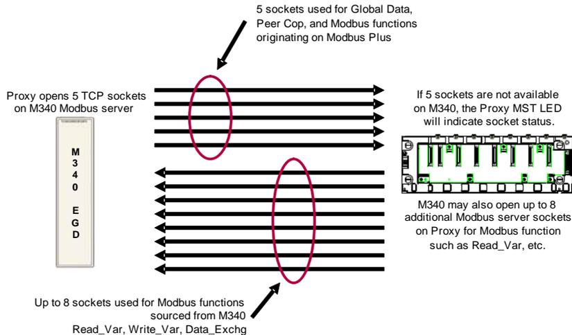
**NOTE:** The M340 supports more than 8 Modbus server sockets, but processes only 8 transactions per CPU scan.
