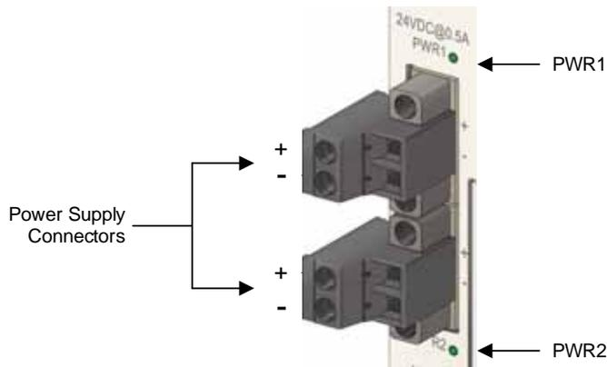
**NOTE:** Refer to the power supply LED diagnostic table (*see page 60*) for a list of power supply LED connector diagnostic codes.
