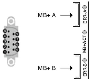
The connectors include one LED (MB+ACT) indicating network status and two LEDs (ERR-A and ERR-B) indicating communication status. For a list of Modbus Plus diagnostic codes, refer to the Modbus Plus LED diagnostic table (*see page 59*).
