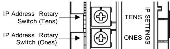
**NOTE:** If you are required to change the IP address settings, the M340 EGD must be rebooted for the changes to take effect.
