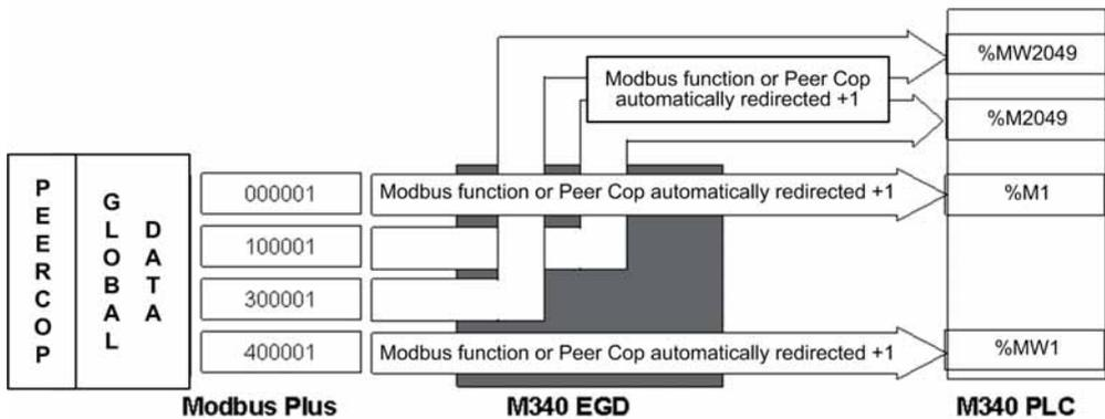
**NOTE:** Modbus function and Peer Cop messages are automatically redirected +1 to accommodate the difference in starting registers for a converted 984 programming application.
