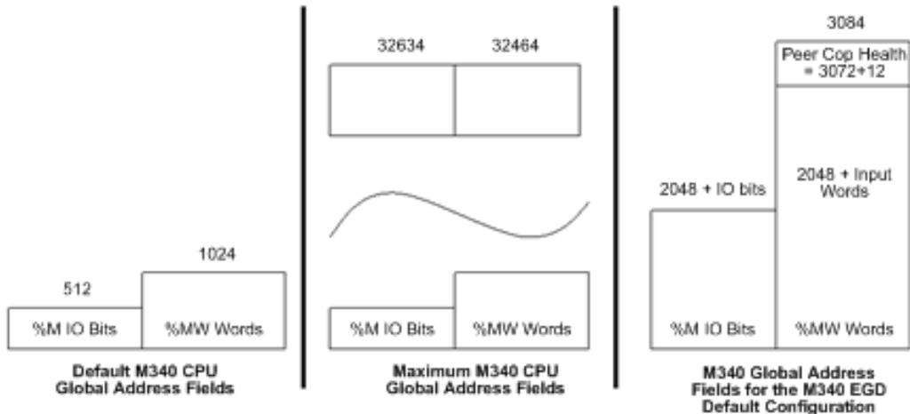
Peer Cop Health writes 12 words to the M340 CPU starting by default at %MW3072. To accommodate the Health block at this default location, configure the CPU for a minimum of %MW3084 words. If these 12 words are not configured in the CPU and reserved for the Health block, Peer Cop and Global Data services are disabled on Modbus Plus.
