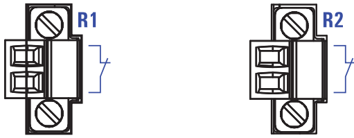
Figure 3: Pin assignment of the signal contact
