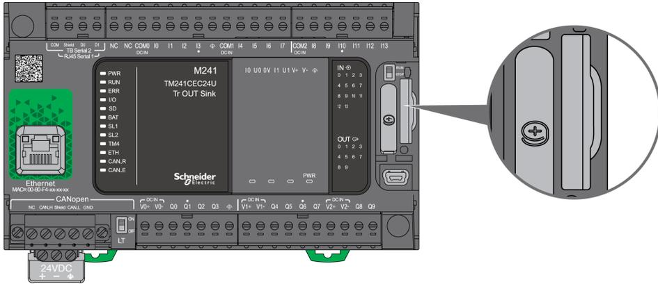
It is possible to set the Write-Control Tab to prevent write operations to the SD card. Push the tab up, as shown in the example on the right-hand side, to release the lock and enable writing to the SD card. Before using an SD card, read the manufacturer's instructions.
