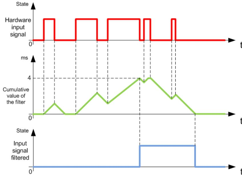
**NOTE:** The value selected for the filter's time parameter specifies the cumulative time in ms that must elapse before the input can be 1.
