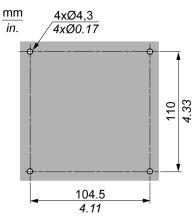
Verify that the installation panel or cabinet surface is flat (planarity tolerance: 0.5 mm (0.019 in)), in good condition, and has no jagged edges.
