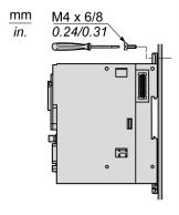
If mounting the controller on a horizontal metallic panel, use flat head screws.
