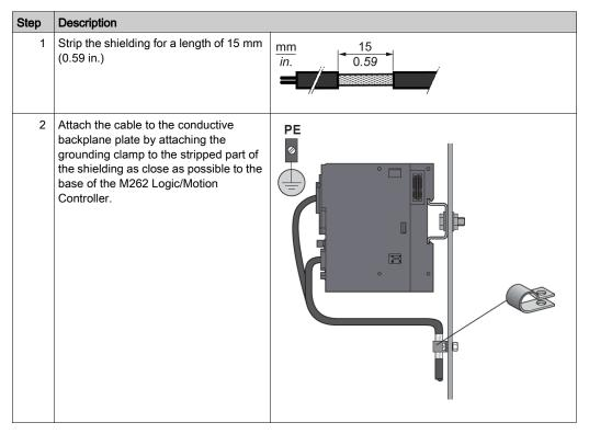
**NOTE:** The shielding must be clamped securely to the conductive backplane to help ensure good contact.
