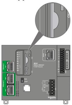
It is possible to set the Write-Control Tab to prevent write operations to the SD card. Push the tab up, as shown in the example on the right-hand side, to release the lock and enable writing to the SD card. Before using an SD card, read the manufacturer's instructions.
