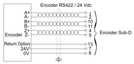
The following illustration describes the wiring diagram of an incremental encoder (RS422 / 5 Vdc or push-pull) mounted on the encoder interface:
