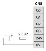
\* Use a type T fuse appropriate for the load, not to exceed 2.5 A
