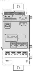
NOTE: TM3 expansion modules must be mounted above the controller.
