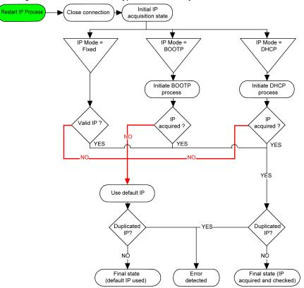
**NOTE:** If a device programmed to use the DHCP or BOOTP addressing methods is unable to contact its respective server, the controller uses the default IP address. It repeats its request constantly.
