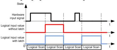
The following timing diagram illustrates the latching effects:
