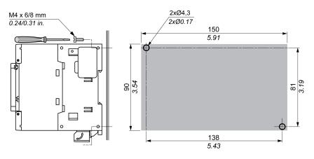
The following diagram shows the mounting hole layout for M241 Logic Controller with 40 I/O channels:
