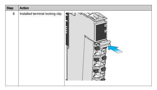
NOTE: To remove the terminal block, reverse Step 5 by pulling out the terminal locking clip.
