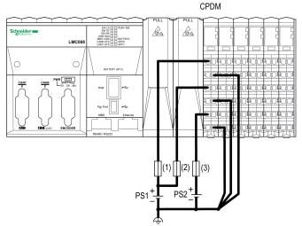
The following figure shows a CPDM wired with two separate external 24 Vdc power supplies:
