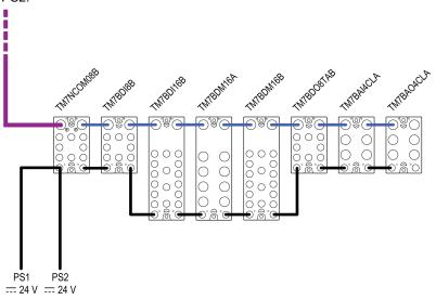
PS1 External isolated main power supply, 24 Vdc
