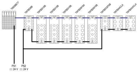
**PS1** External isolated main power supply, 24 Vdc **PS2** External isolated I/O power supply, 24 Vdc
