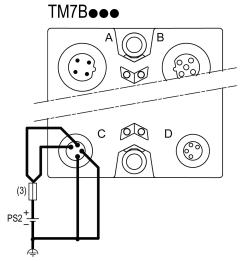
(3) External fuse, Type T slow-blow, 8 A maximum, 250 V PS2 External isolated I/O power supply, 24 Vdc
