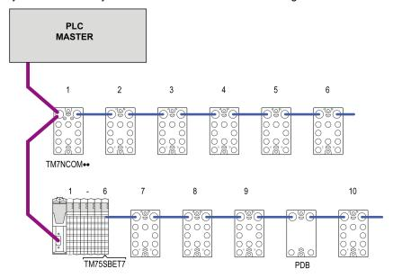
TM7NCOM •• TM7 Field bus interface I/O block
