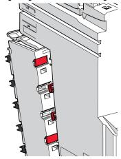
The label tabs and labeling tool *(see page 59)* accessories are required to code the terminal block and the electronic module.
