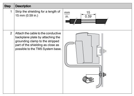
**NOTE:** The shielding must be clamped securely to the conductive backplane to help ensure good contact.
