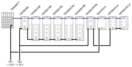
**PS1** External isolated main power supply, 24 Vdc **PS2** External isolated I/O power supply, 24 Vdc
