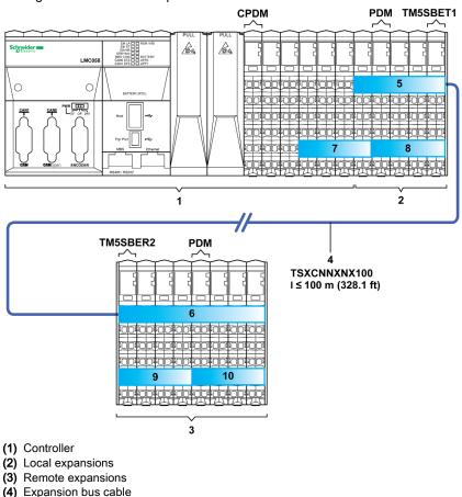
The figure below shows the power distribution overview of local and remote configurations:
