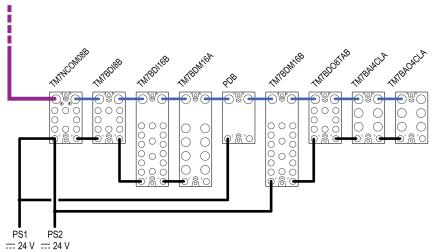
**PS1** External isolated main power supply, 24 Vdc **PS2** External isolated I/O power supply, 24 Vdc
