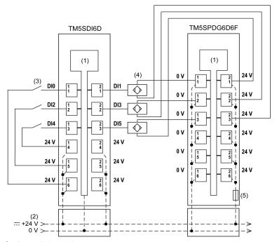
The following figure shows the wiring diagram for the TM5SPDG6D6F with a TM5SDI6D:
