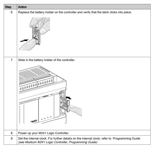
**NOTE:** Replacement of the battery in the controllers other than with the type specified in this documentation may present a risk of fire or explosion.
