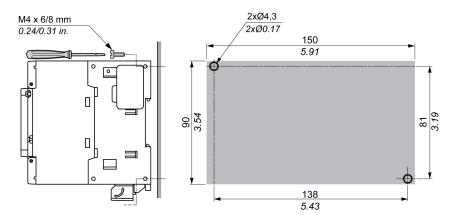
The following diagram shows the mounting hole layout for M241 Logic Controller with 40 I/O channels:
