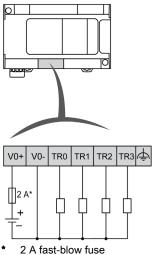
Fast output wiring for TR0... TR3:
