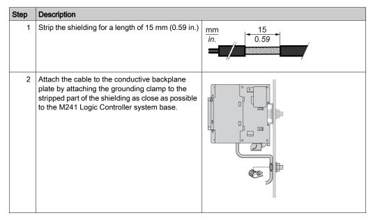
**NOTE:** The shielding must be clamped securely to the conductive backplane to ensure a good contact.
