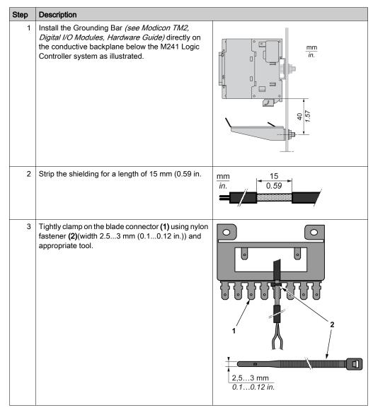
**NOTE:** Use the TM2XMTGB Grounding Bar for Functional Ground (FE) connections.
