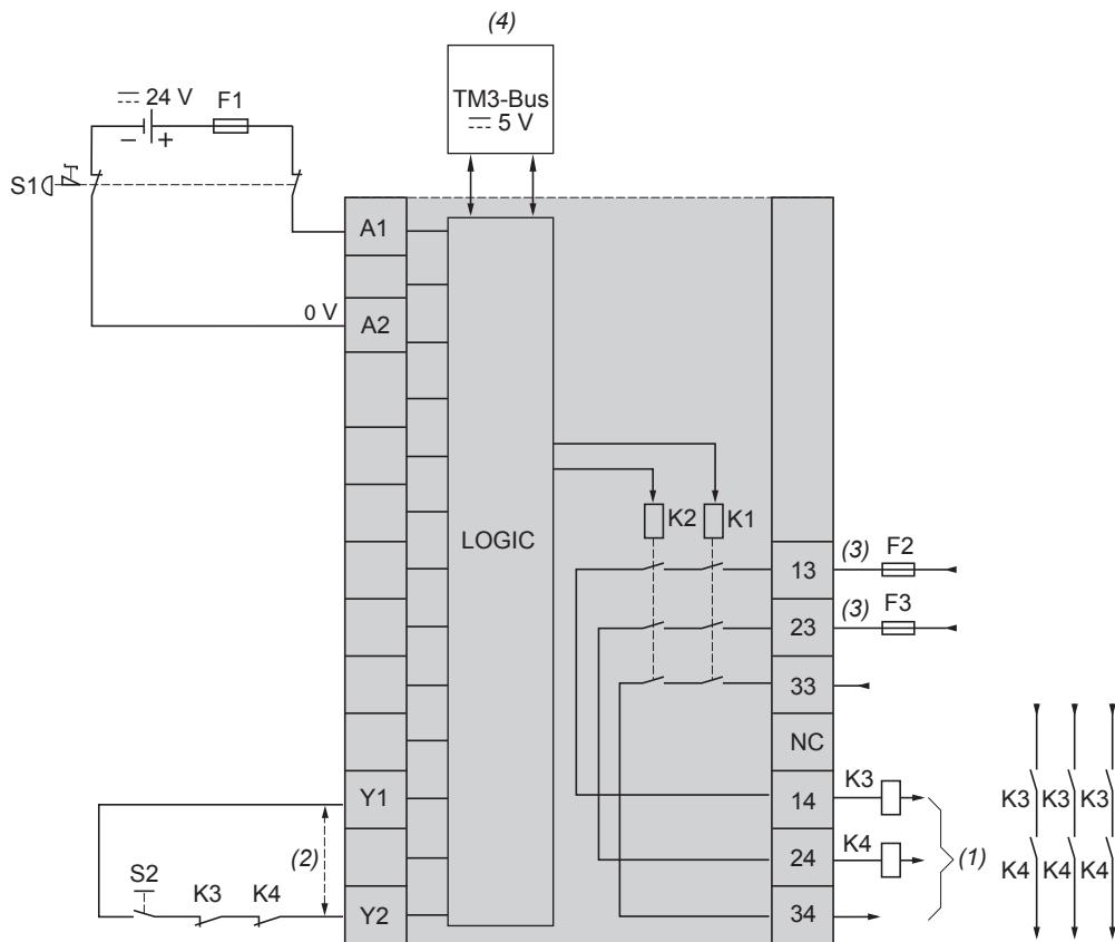
S1= EMERGENCY STOP / Bouton poussoir d'ARRÊT D'URGENCE / Not-Halt / PARADA DE EMERGENCIA / ARRESTO DI EMERGENZA / 紧急停止.
