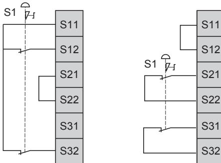
**Note:** Inputs S11 and S12 are not intended for the monitoring of short circuits in external wiring.
