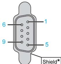
\* To be connected externally to the protective earth
