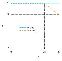
% Simultaneity factor°C Ambient temperature
