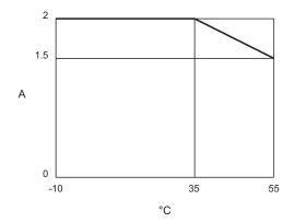
If the dissipation restriction of adjacent modules is not possible in your configuration, the de-rating must shift by -5 °C (- 9 °F), and 2 A / output can be maintained at 30 °C (86 °F). In most industrial applications, this would require the module to be in an air conditioned enclosure to maintain such temperatures.
