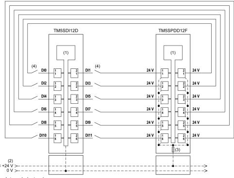
The following illustration shows the wiring diagram for the TM5SPDD12F and a TM5SDI12D:
