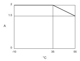
If the dissipation restriction of adjacent modules is not possible in your configuration, the de-rating must shift by -5  $^{\circ}$ C (- 9  $^{\circ}$ F), and 2 A / output can be maintained at 30  $^{\circ}$ C (86  $^{\circ}$ F). In most industrial applications, this would require the module to be in an air conditioned enclosure to maintain such temperatures.
