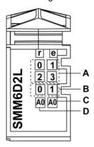
The table shows the TM5SMM6D2L input status LEDs:
