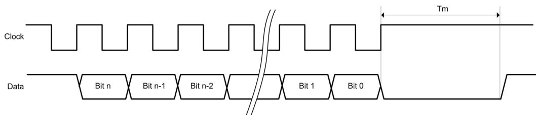
In the example 2 the **Monoflop check** parameter must be configured to low level. This ensures that the clock generation is postponed until the data line goes low.
