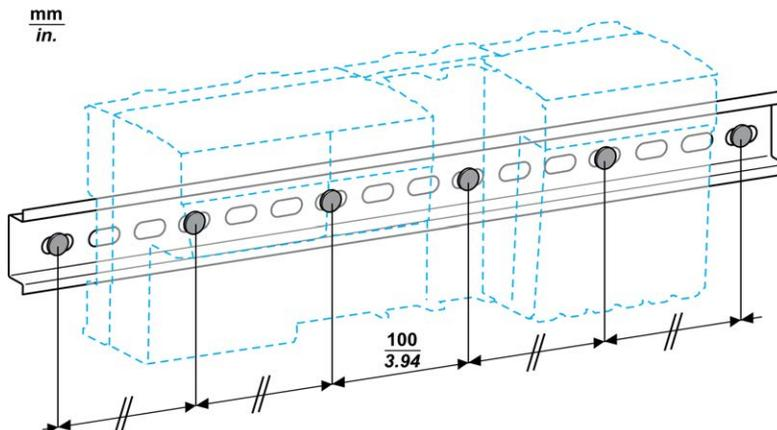
Low profile NSYSR200D DIN rail may be used with low profile mounting hardware such as flat head screws with countersunk mounting holes.
