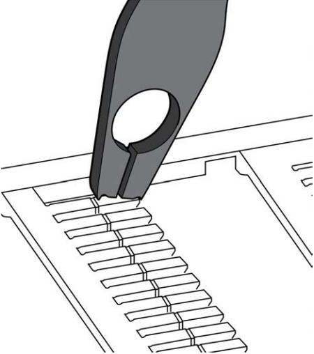
A line drawing of a terminal block with a locking clip. A labeling tool with a circular hole and a narrow cutting edge is shown gripping a small tab on one of the terminals. The tool is positioned vertically, with the cutting edge pointing downwards into the tab. |
