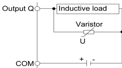
In applications where the inductive load is switched on and off frequently and/or rapidly, ensure that the continuous energy rating (J) of the varistor exceeds the peak load energy by 20% or more.
