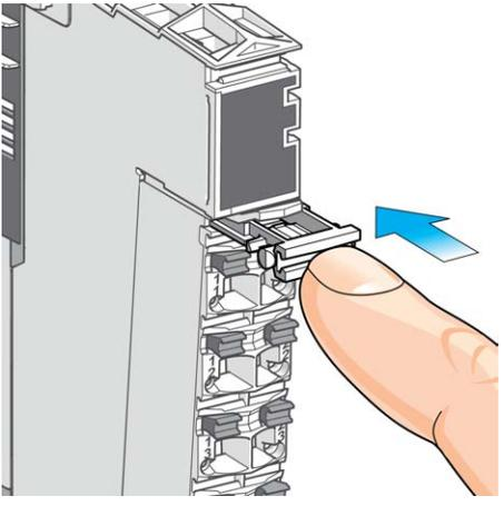
A technical illustration showing a finger pushing a locking clip into the terminal block. The clip is shown in a position where it will engage with the terminals. A blue arrow points to the right, indicating the direction of the push.       |
