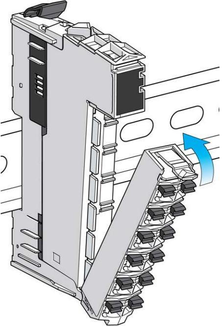
A technical illustration of a terminal block being rotated into place. The block is shown at an angle, with a blue arrow indicating the direction of rotation. The block is being moved towards a set of terminals on a larger electronic module. |
