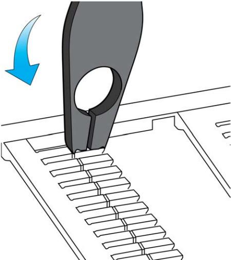
A line drawing of the same terminal block and labeling tool. A blue curved arrow points downwards from the tool, indicating the direction of pressure. The tool is now shown pressing down on the tab, which is beginning to separate from the terminal block.         |
