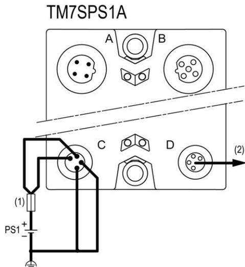
(1) External fuse, Type T slow-blow, 1 A minimum, 4 A maximum, 250 V
