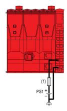
(1) External fuse, Type T slow-blow, 1 A, 250 V **PS1** External isolated power supply 24 Vdc
