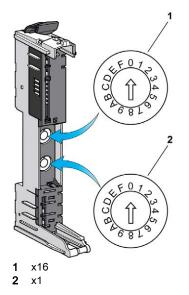
The address of the slice is set using the address setting rotary switches (01 - FD hex).
