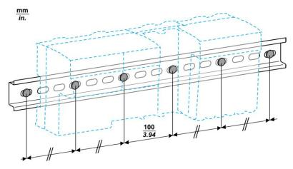
Low profile NSYSDR200D DIN rail may be used with low profile mounting hardware such as flat head screws with countersunk mounting holes.
