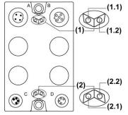
(1) TM7 power bus status LEDs, set of two LEDs: 1.1 (green) and 1.2 (green)
