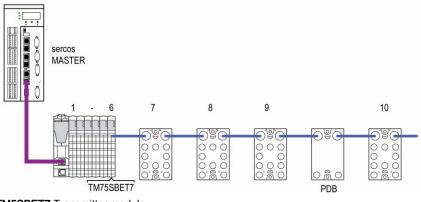
**TM5SBET7** Transmitter module **PDB** Power Distribution Block
