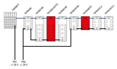
**PS1** External isolated main power supply, 24 Vdc **PS2** External isolated I/O power supply, 24 Vdc
