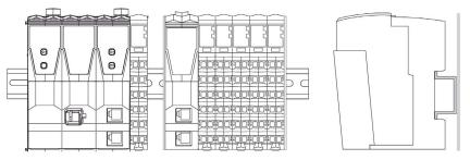
**NOTE:** The Safety Controller TM5CSLC100FS/TM5CSLC200FS can only be connected with the safety-related modules via the Sercos III Bus Interface TM5NS31. There is no electrical connection between Safety Controllers and the safety-related modules via the bus base.
