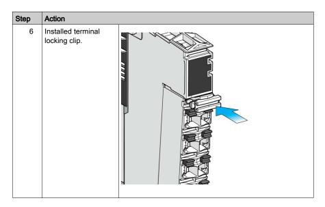
NOTE: To remove the terminal block, reverse Step 5 by pulling out the terminal locking clip.
