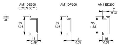
NOTE: Only size 1 (smallest) blocks can be installed on DIN rail with the mounting plate.
