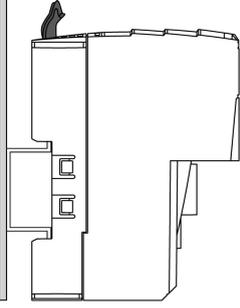
A line drawing of a control panel being inserted into a vertical mounting rail. The panel has a top edge with a hook-like structure that fits into the rail. The panel is shown from a side-on perspective, with its front face facing right. |
