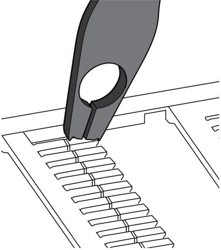
A line drawing of a terminal block with multiple terminals. A labeling tool, which has a circular hole and a pointed tip, is shown gripping one of the terminals. The tool is positioned vertically, with its tip resting on the terminal.                                                             |
