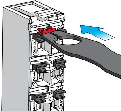
A technical diagram of a terminal block with a labeling tool. The tool is a grey, curved piece with a red tab. A blue arrow points from the right towards the tool, indicating the direction of movement to center it over a slot. The terminal block has several rows of terminals, with the top row being the focus. The tool is positioned over a slot in the top row. |
