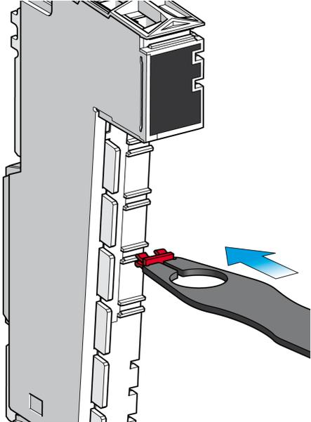
A technical diagram of an electronic module with a vertical row of slots. A labeling tool with a red tip and a grey handle is shown pressing a label tab into one of the slots. A blue arrow points to the right, indicating the direction of the force applied by the tool. |
