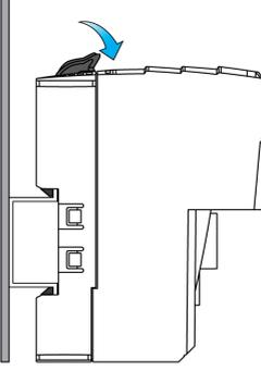
A line drawing of the control panel mounted on the rail. A blue arrow points to a lever on the top edge of the panel, indicating it should be pushed down. The panel is shown from a side-on perspective, with its front face facing right.   |
