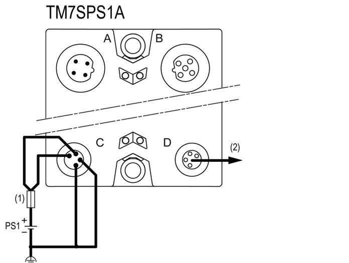
(1) External fuse, Type T slow-blow, 1 A minimum, 4 A maximum, 250 V
