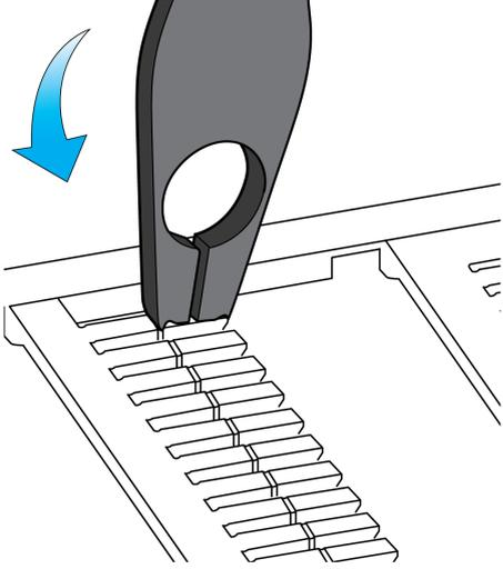
A line drawing of the same terminal block and labeling tool as in the previous diagram. A blue curved arrow indicates the tool is being pressed down onto the terminal. The tool's tip is now fully seated on the terminal, and the label tab is being separated from the rest of the terminal block. |
