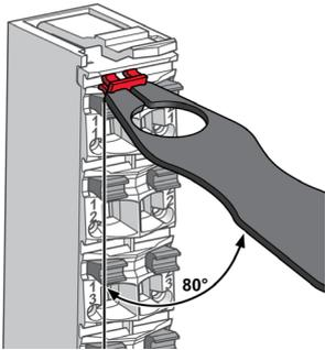
A technical diagram of the same terminal block and labeling tool. The tool is now held at an angle to the terminal block. A curved arrow indicates the angle, which is labeled as 80°. The red tab of the tool is now positioned over the slot in the top row of the terminal block.                                                                                      |
