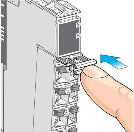
A close-up technical illustration of the terminal block assembly. A human finger is shown pushing a small, rectangular locking clip into a slot on the side of the terminal block. A blue arrow points to the right, indicating the direction of the push.                                            |
