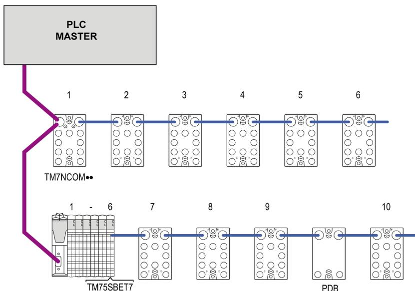
**TM7NCOM\*\*** TM7 Field bus interface I/O block
