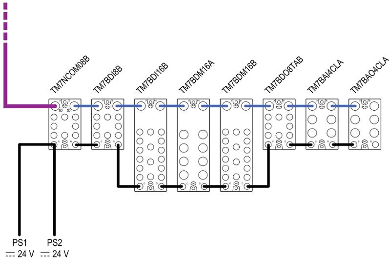
**PS1** External isolated main power supply, 24 Vdc
