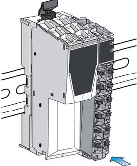
A technical line drawing of a fieldbus interface unit. The unit is rectangular with a hinged door on the left side. On the right side, there is a vertical mounting rail with several slots. A blue arrow points to a lever mechanism at the bottom of the rail, which is used to lock the interface into place. Wires are shown entering and exiting the unit from both sides. |
