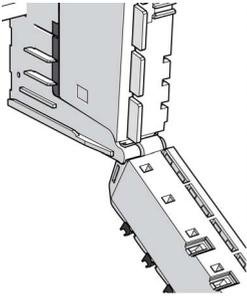
A technical drawing showing a terminal block being positioned to be hung on a bus base. The terminal block is tilted downwards, and its bottom edge is being aligned with the bus base.                                            |
