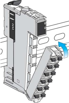
A technical drawing showing the terminal block being rotated upwards. A blue curved arrow indicates the direction of rotation. The terminal block is now more vertical, and its bottom edge is being pushed towards the bus base. |
