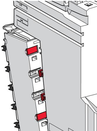
The label tabs and labeling tool ([see page 52](#)) accessories are required to code the terminal block and the electronic module.
