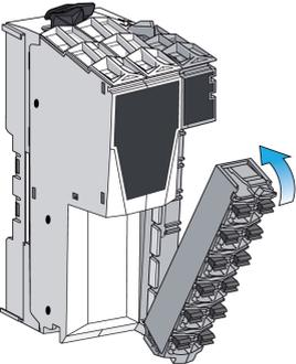
A technical illustration showing the terminal block rotated upwards from its previous position. A blue curved arrow indicates the direction of rotation.                                                                                                                  |
