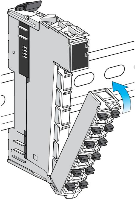
A technical line drawing of a terminal block being rotated into place. The block is shown at an angle, with a blue curved arrow indicating the direction of rotation. The block is being moved towards a larger electronic module.         |
