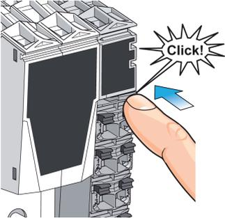
A technical illustration showing a hand pushing the terminal block into the bus base. A blue arrow points to the terminal block, and a starburst graphic with the word "Click!" indicates the sound of the block locking into place.                                     |
