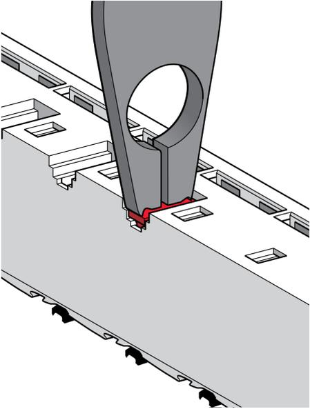
A 3D cutaway diagram of a terminal block. A grey labeling tool with a circular hole is positioned over a red label tab. The tool is being used to push the tab into a slot on the back of the terminal block. The terminal block is shown in a perspective view, with several other slots visible along its length.      |
