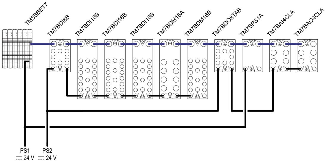
**PS1** External isolated main power supply, 24 Vdc
