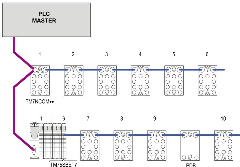
**TM7NCOM** TM7 Field bus interface I/O block
