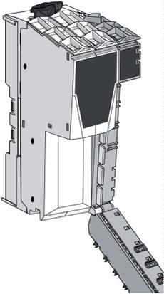
A technical illustration showing a grey terminal block being aligned with a bus base. The bottom edge of the terminal block is being inserted into a hinge on the bus base. A screwdriver is shown at the top of the terminal block, indicating it is being held in place. |
