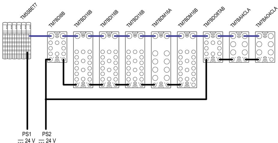
**PS1** External isolated main power supply, 24 Vdc
