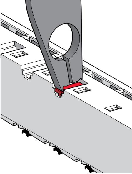
A 3D cutaway diagram of a terminal block, similar to the one in step 6. The red label tab is now fully seated in the slot. The grey labeling tool is being used to push the left feet of the label into the slot. The terminal block is shown in a perspective view, with several other slots visible along its length. |
