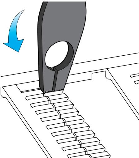
A technical line drawing of the same terminal block and labeling tool. The tool is now pressed down against the top of the label tab. A blue curved arrow on the left side of the tool indicates the downward direction of the applied force. |
