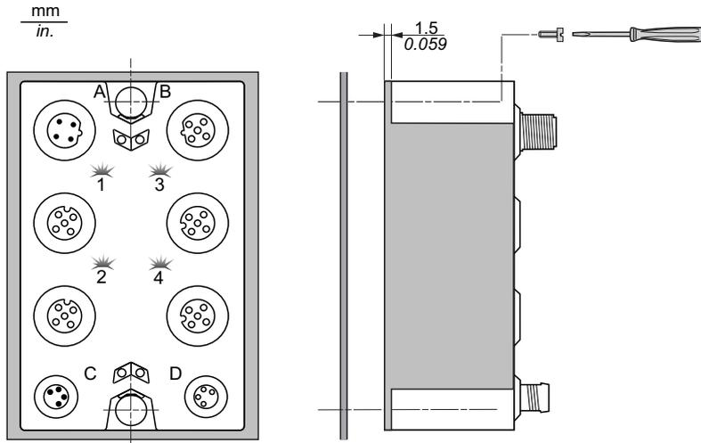
**NOTE:** Maximum torque to fasten the required M4 screws is 0.6 Nm (5.3 lbf-in).
