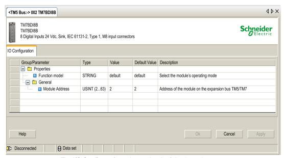
The I/O Configuration tab contains the following columns:
