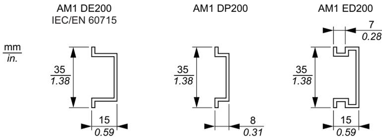
**NOTE:** Only size 1 (smallest) blocks can be installed on DIN rail with the mounting plate.
