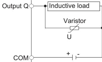
In applications where the inductive load is switched on and off frequently and/or rapidly, ensure that the continuous energy rating (J) of the varistor exceeds the peak load energy by 20% or more.
